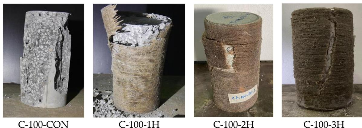
**Figure 7.** Failure modes of concrete prisms (Group 3).
