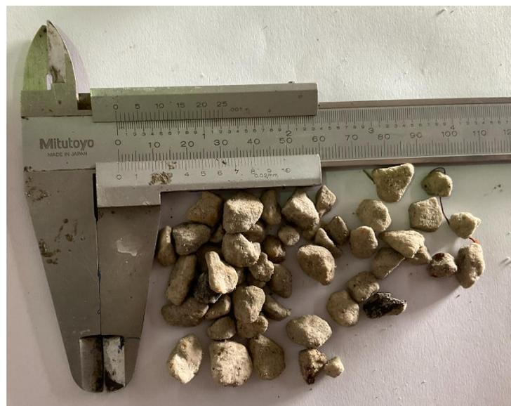
**Figure 1.** Lightweight aggregates.
