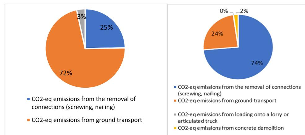
**Figure 9.** CO<sub>2</sub>e,1 emissions from the demolition activity for Villa GP (left) and the Via Cenni complex (right).
