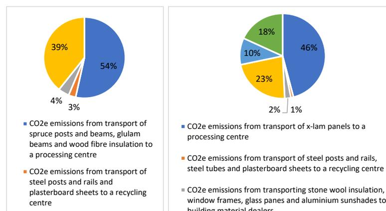
**Figure 11.** CO<sub>2</sub>e,3 emissions from off-site transport for Villa GP (left) and Via Cenni complex (right).
