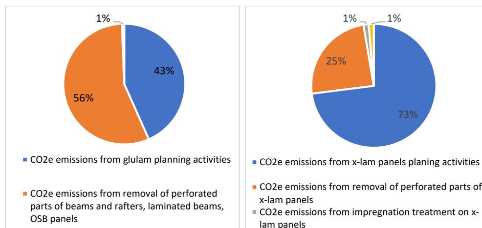
**Figure 12.** CO<sub>2</sub>e,4 emissions from transformation/treatment for further reuse for Villa GP (left) and the Via Cenni complex (right).
