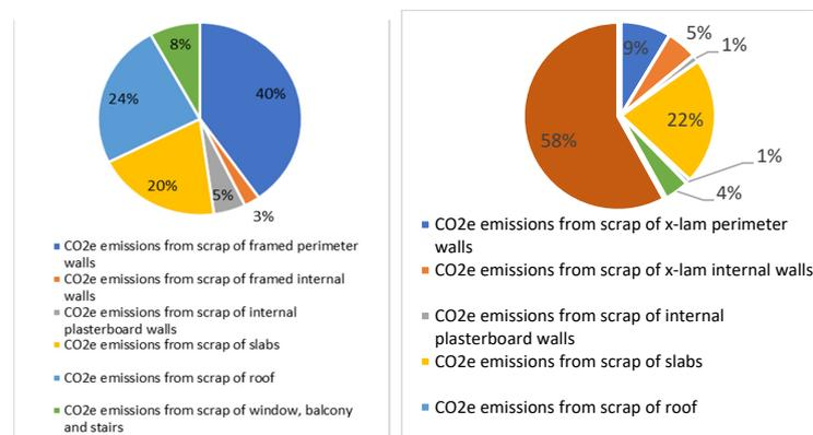
**Figure 10.** CO<sub>2</sub>e,2 emissions from scrap resulting from demolition operations for Villa GP (left) and the Via Cenni complex (right).
