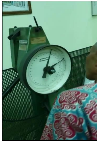
Figure 7. Impact testing process.
