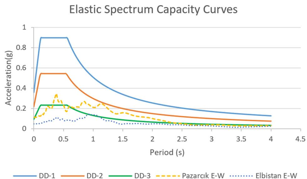
**Figure 13.** Comparison of the spectral acceleration and specification elastic spectrum capacity values of the station 2107 in Diyarbakır province.
