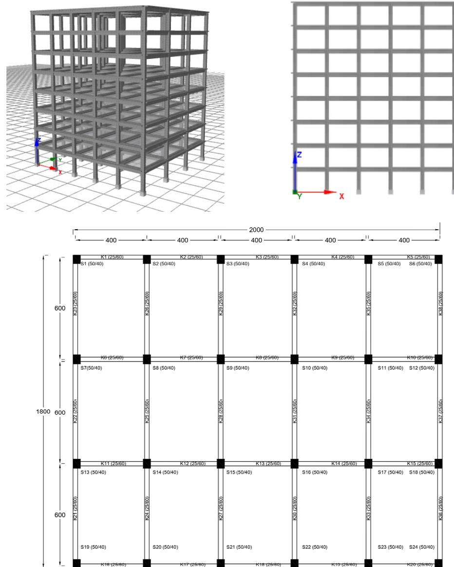
Figure 12. 2D and 3D views with blueprint of the sample RC model.
