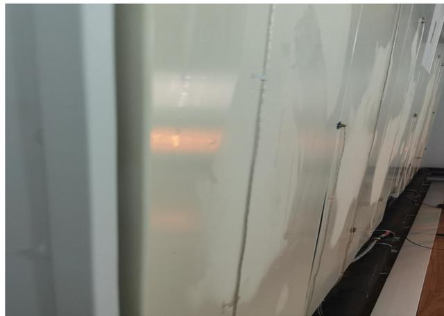
**Figure 16.** Radiation-cold-plate surface condensation. Diameter of condensation droplets is between 1 mm and 3 mm.
