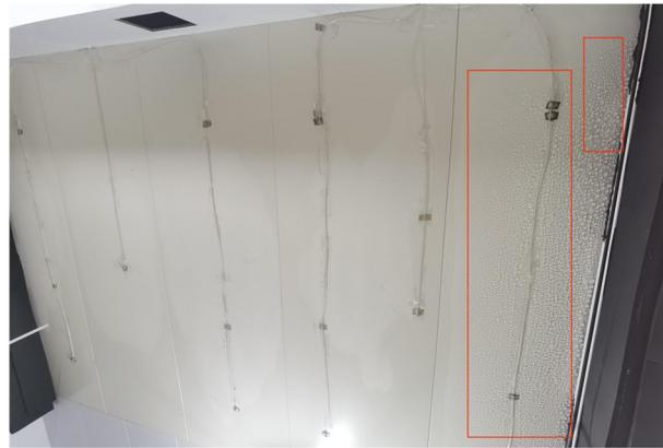
**Figure 21.** Radiation-cold-plate surface condensation. Diameter of condensation droplets is between 1 mm and 7 mm.
