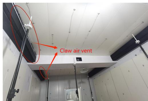
**Figure 4.** Physical diagram of the radiant roof combined with adherent-jet air conditioning system.
