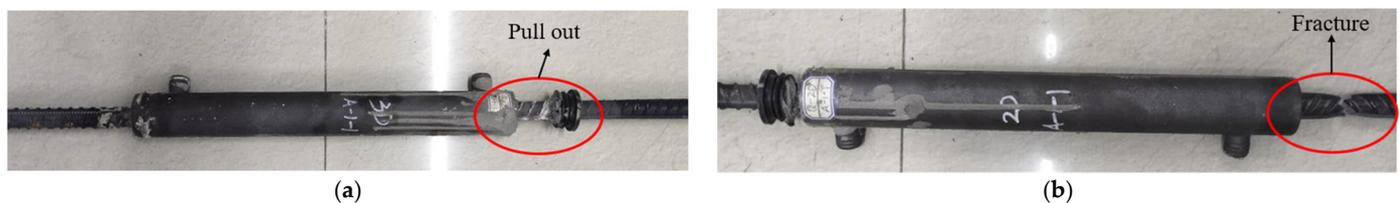
**Figure 7.** Failure modes: (a) steel bar pullout failure; (b) steel bar fracture failure.
