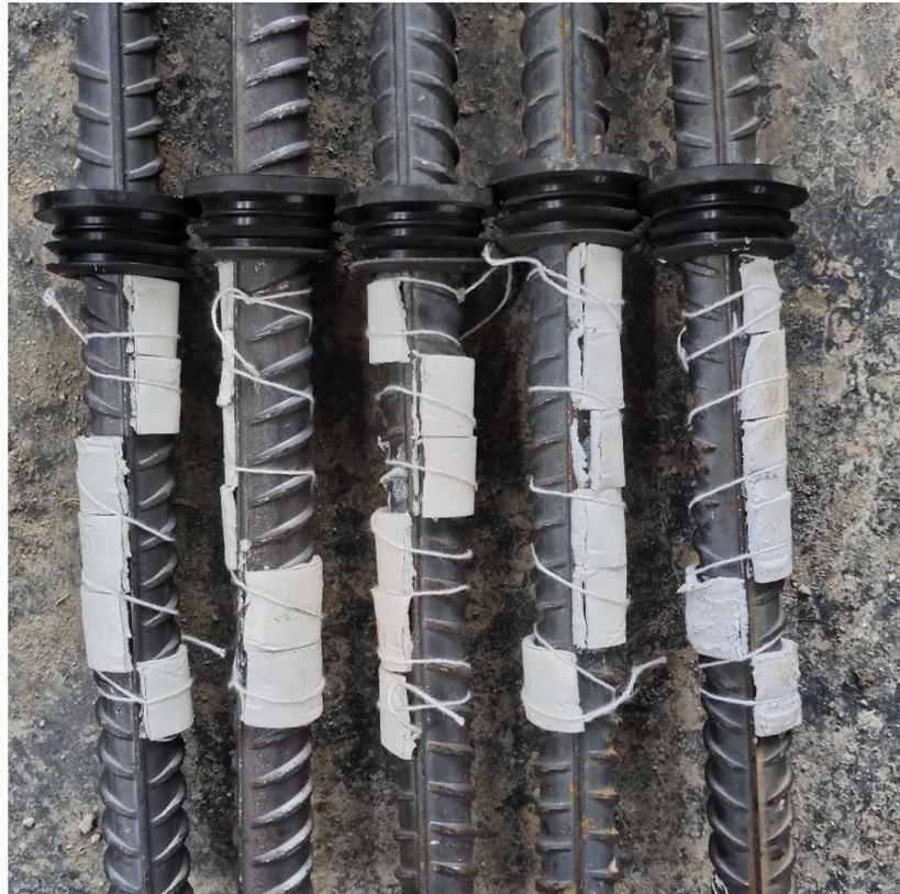
**Figure 4.** Defect settings of piles.
