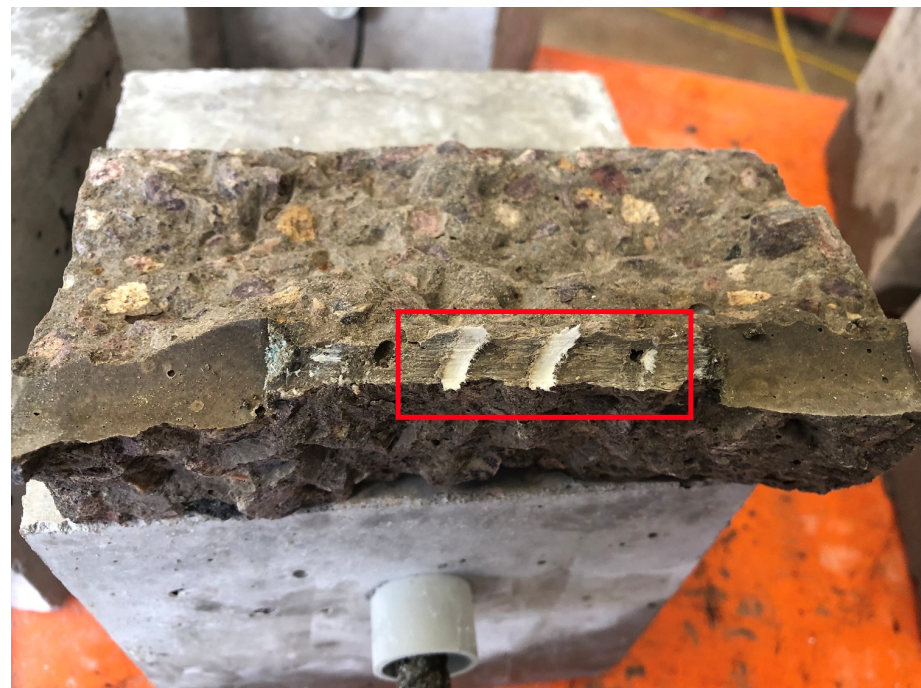
Figure 9. Ribbed impression highlighted on split concrete in pull-out test for a GFRP ribbed bar.
