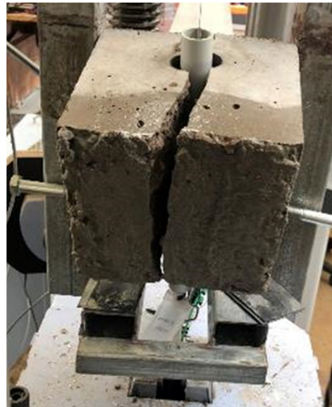
Figure 8. Example of concrete split failure observed for pull-out tests for ribbed rebar.
