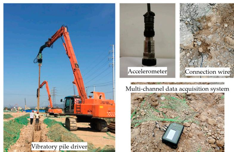
**Figure 3.** Test site setup.
