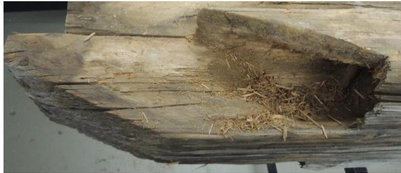
**Figure 13.** Damage to the beam (H2) in the location of the dovetail joint.
