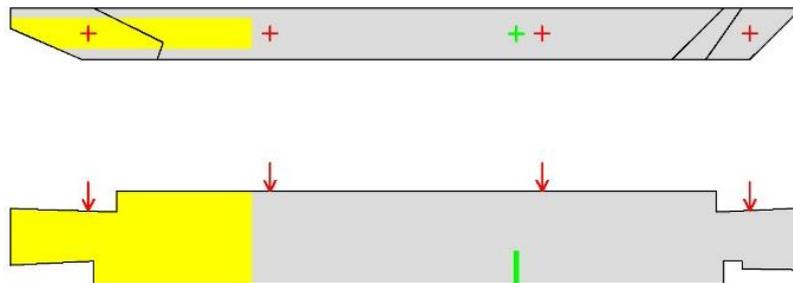
**Figure 14.** A scheme of the extent of rot, beam (H2) (yellow—replacement, grey—standard wood density without need of repair). Arrow and + marking points measured with Resistograph.
