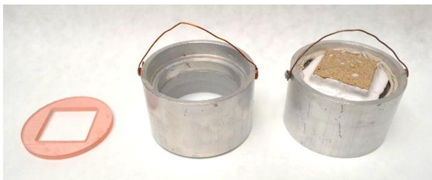
**Figure 35.** Arrangement of the water vapour permeability test.
