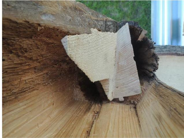
**Figure 18.** The rear insert fixed in the grooves.
