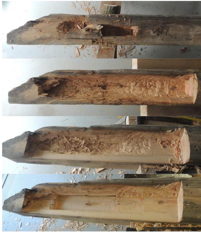
Figure 28. The gradual formation of the bed for the insert copying the damage area.
