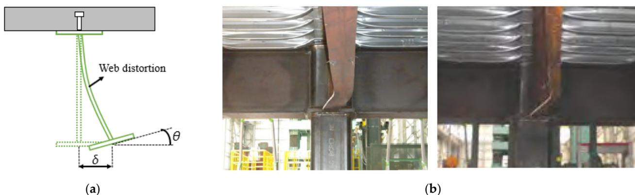
**Figure 5.** Lateral distortional buckling in steel-concrete composite beams: (a) Cross-section behavior (Adapted from Rossi et al. [16]); (b) Experimental tests by Kitaoka et al. [35].
