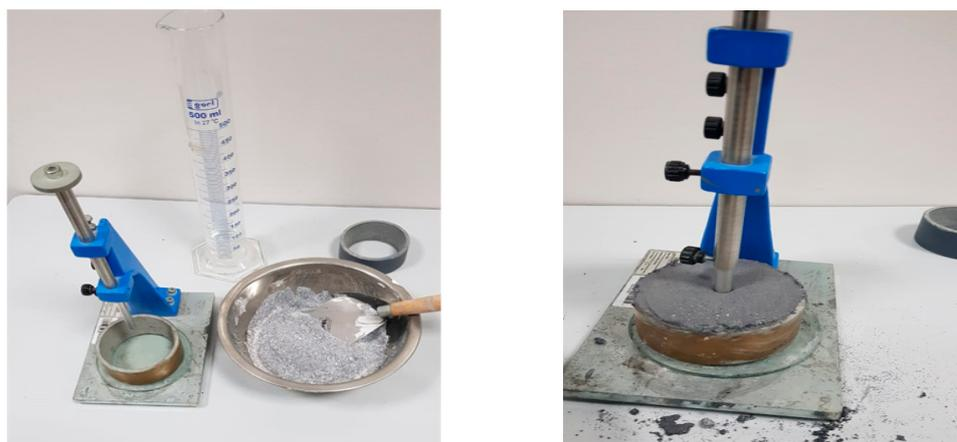
**Figure 5.** Geopolymer paste preparation for normal consistency test.
