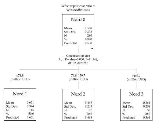
Figure 2. Decision tree of defect repair cost ratio to construction cost.
