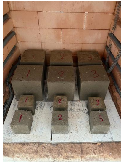
Figure 4. Placement of the specimens in the electric furnace.
