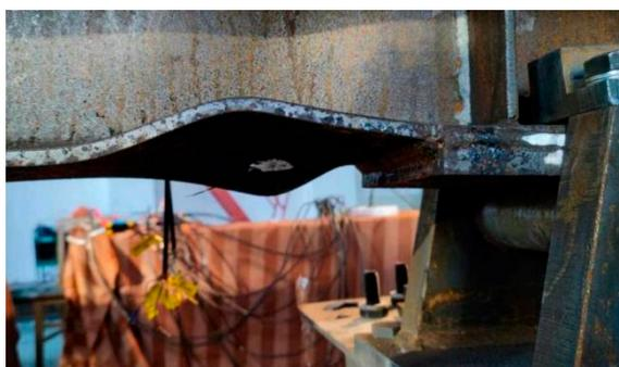
**Figure 8.** Buckling of the bottom flange of CSB-1.
