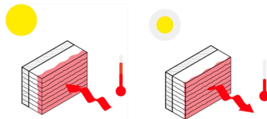
**Figure 2.** Effect of heating and cooling through thermal mass (own representation).
