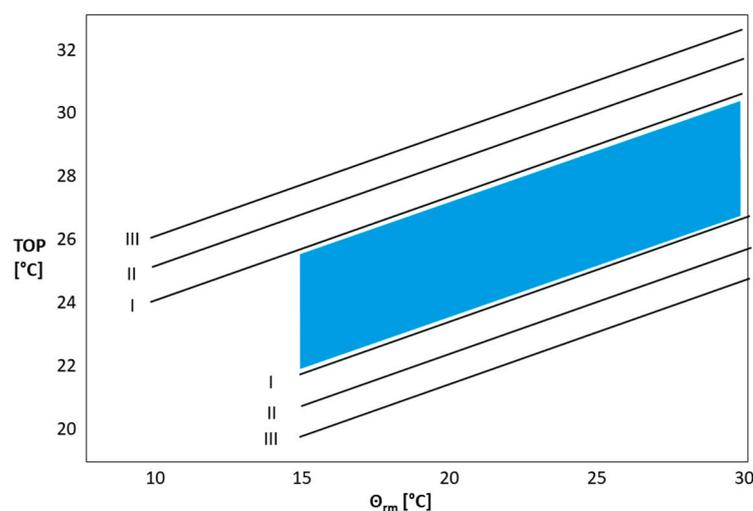
**Figure 3.** Energy saving potential within the adaptive thermal comfort band (own representation based on DIN EN 16798-1 [22]).
