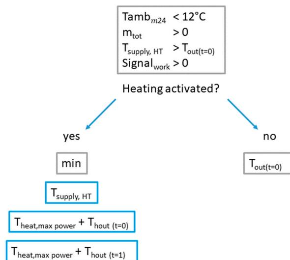
**Figure 6.** Heating scheme set-up (own representation).
