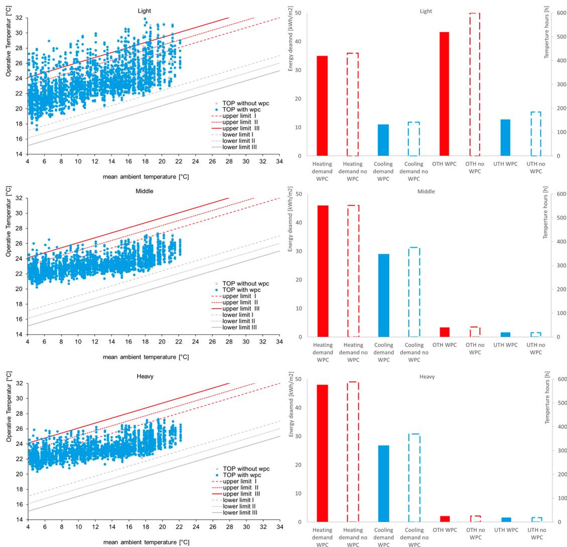
**Figure 8.** Simulation Results: Left column: Comfort hours with (blue) and without WPC (grey) for a lightweight (top), middle (middle) and heavy (bottom) construction; right column: Heating (red) and cooling (blue) demand and over (red) and under temperature hours (blue) with (solid color) and without (dashed) WPC (own representations).
