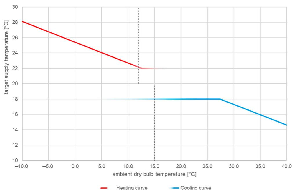
**Figure 4.** Exemplary heating and cooling curve for TABS (own representation).
