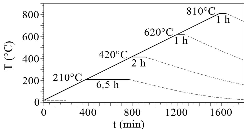
Figure 2. The heating regime of SCC specimens.
