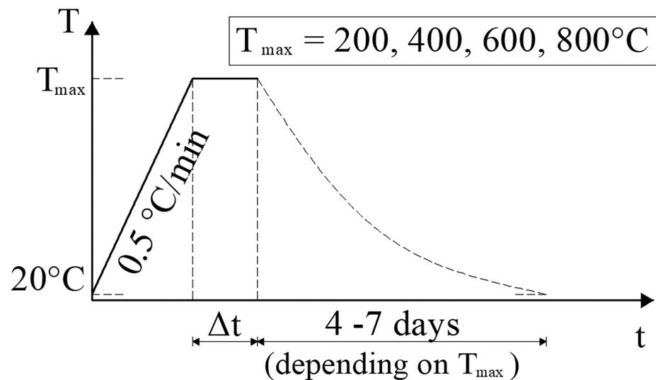
Figure 1. Heating and cooling rates of SCC specimens.
