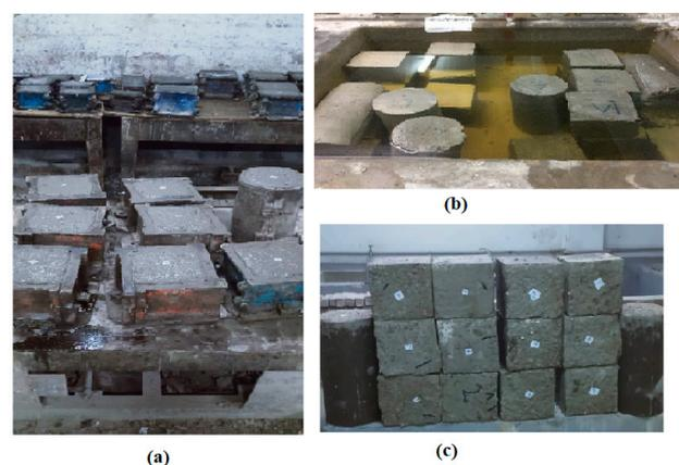
**Figure 3.** Steps of mixing and curing: (a) molding concrete samples; (b) Samples in curing tank; (c) de-molding concrete samples.
