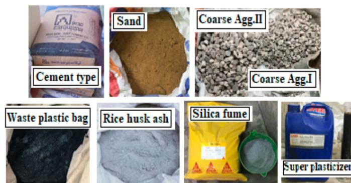
**Figure 2.** Sample of raw materials used in concrete mix.
