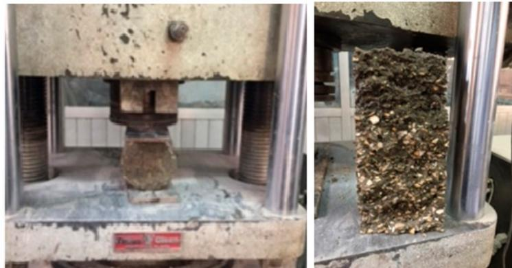
**Figure 4.** Testing of concrete tensile strength with sample of cylinder.
