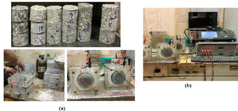
**Figure 6.** Conducting RCP test for concrete mixes: (a) preparing samples for RCPT; (b) RCPT apparatus.
