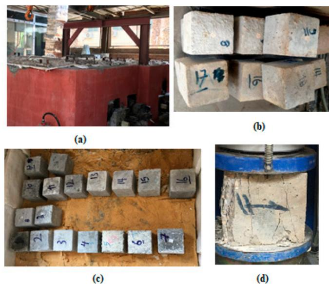
**Figure 7.** Elevated temperature test of concrete specimens: (a) electric furnace device; (b) placing samples in furnace before test; (c) cubic concrete specimens after fire; (d) compressive strength testing after fire.
