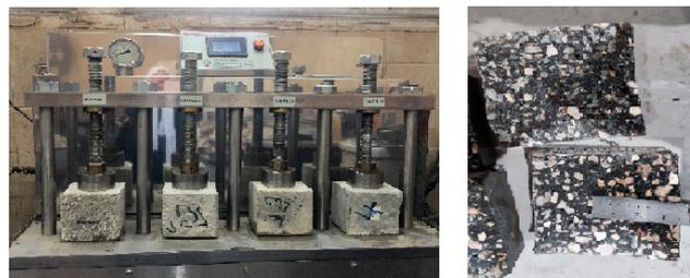
**Figure 5.** Testing of concrete water permeability.
