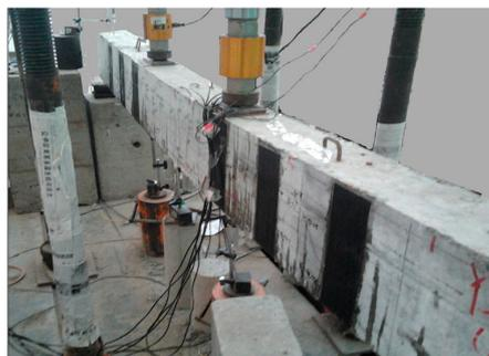
Figure 3. Repeated loading devices for test beams.
