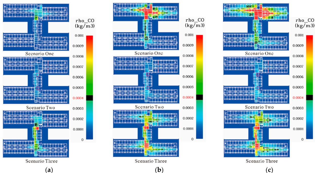
**Figure 5.** Slices of CO concentration at different moments in the ignition layer for different scenarios. (a)  $t = 200$  s. (b)  $t = 400$  s. (c)  $t = 600$  s.
