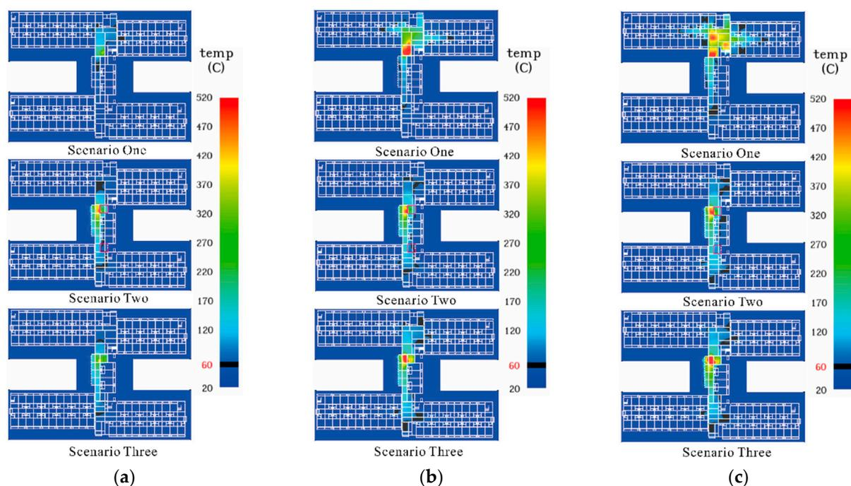
**Figure 4.** Temperature slices of the ignition layer at different moments in time for different scenarios. (a)  $t = 200$  s. (b)  $t = 400$  s. (c)  $t = 600$  s.
