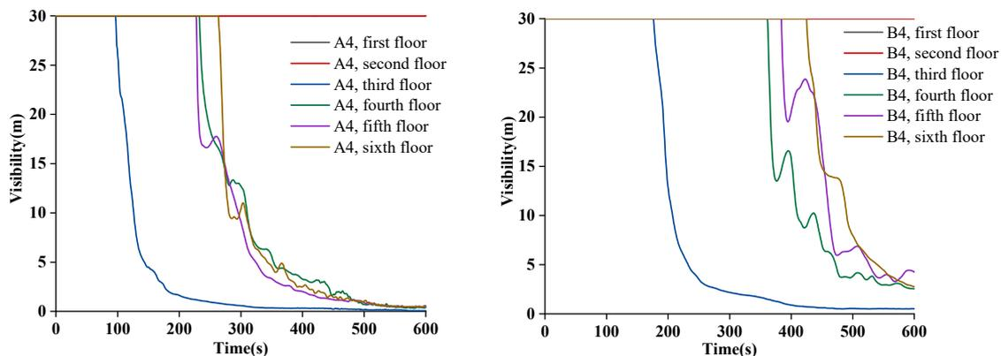
**Figure 7.** Variation of visibility at the vertical detection point in the stairwell.
