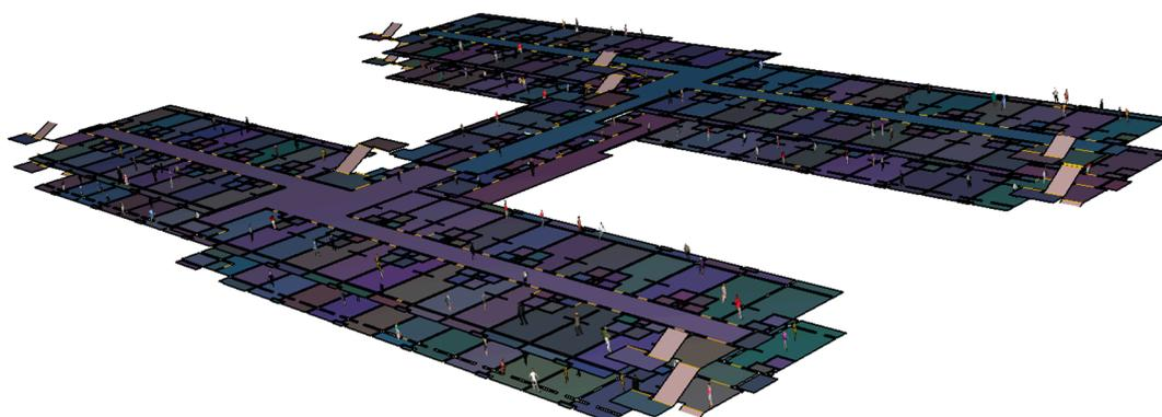
**Figure 10.** Analysis model for egress simulation.
