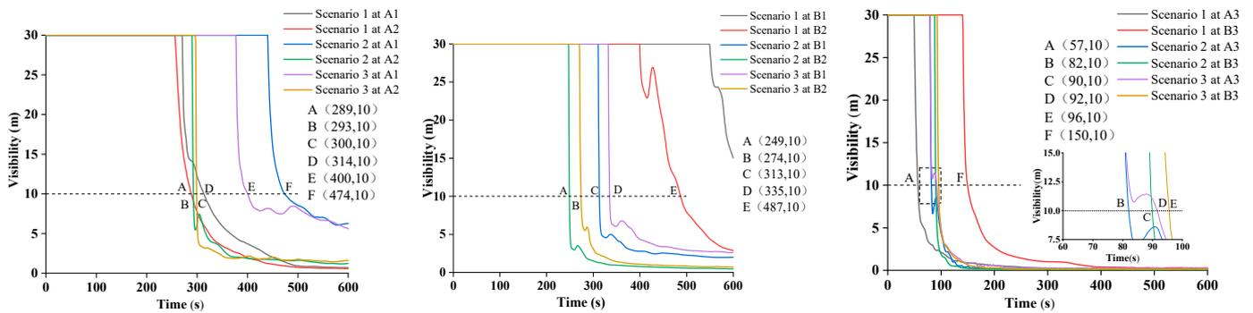
**Figure 9.** Time-visibility variation curves at safety exits for different scenarios.
