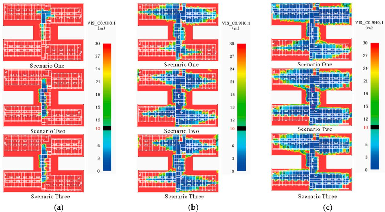
**Figure 6.** Visibility slices at 2 m for different scenarios. (a)  $t = 100$  s. (b)  $t = 300$  s. (c)  $t = 600$  s.
