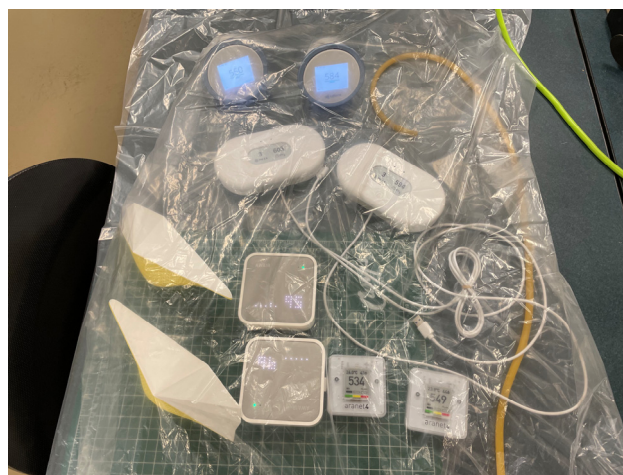
Figure 1. Test devices in the sealed bag during initial CO 2 injection in the lab.
