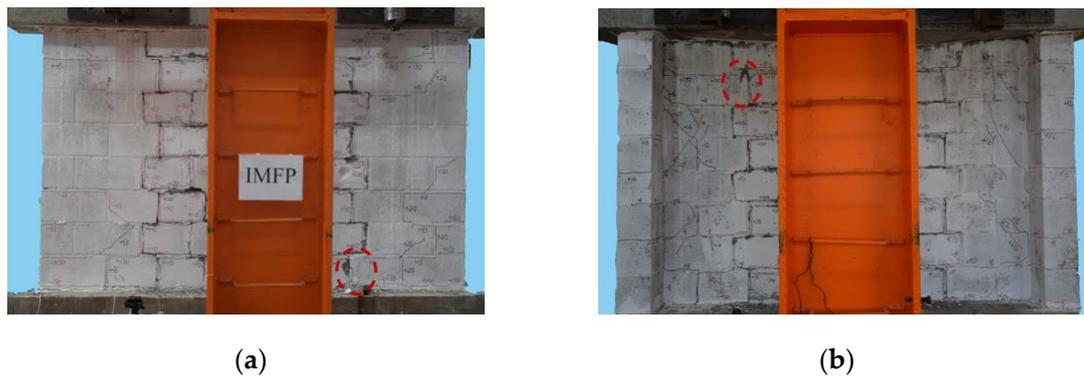
**Figure 9.** Damage state of specimens: (a) specimen IMFP; (b) specimen IMFTP.
