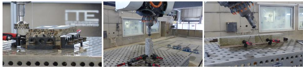
**Figure 14.** Robotic preparation for the attachment of the three types of joints.
