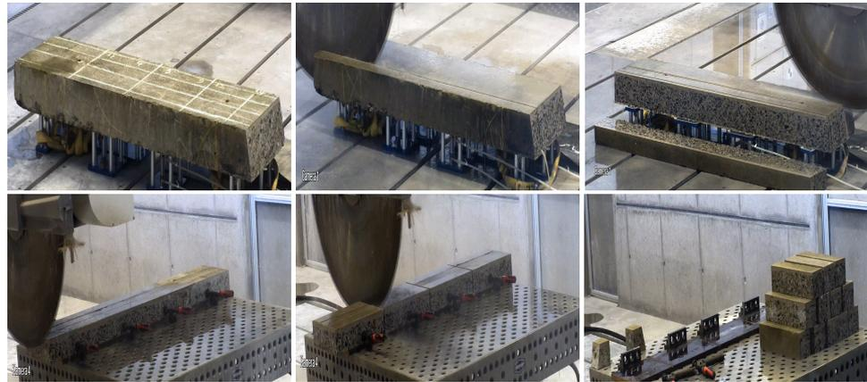
**Figure 13.** Re-utilisation of the concrete floor elements as the beams.
