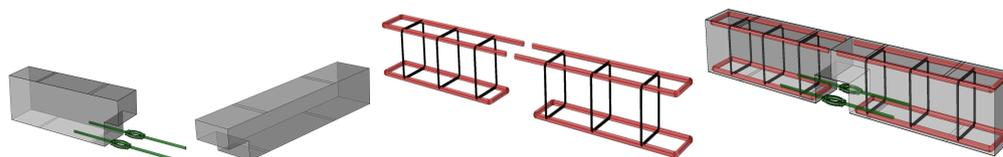
**Figure 3.**  $C_1$ , rebar layout and geometrical dimensions.
