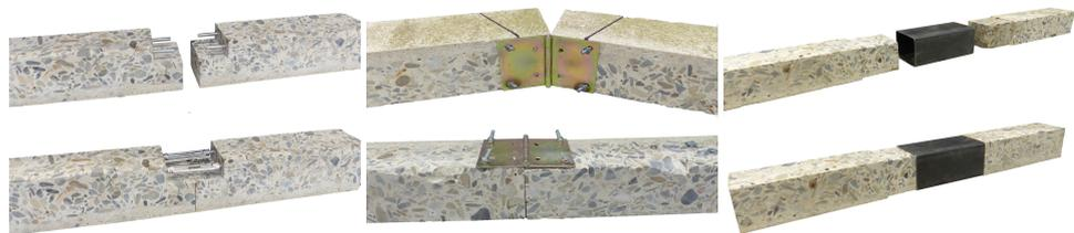
**Figure 15.** Attaching the joints to the re-utilised elements, (Left) coupling connection (C1), (Middle) steel tube connection (C4) (Right) hinge connection (C2).
