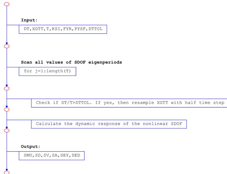
**Figure 2.** Flowchart for the generation of the constant strength response spectrum.
