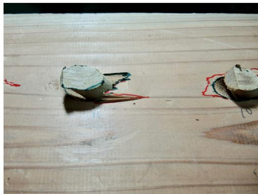
Figure 22. Vacant between A-type dowel and hole.
