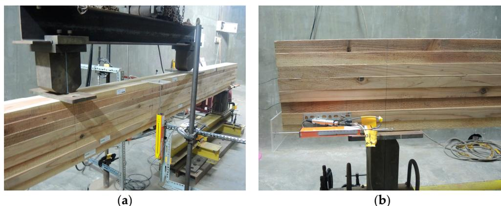
**Figure 4.** Detail of the sensors and specimens. (a) W-shape steel beam and loading points. (b) LVDT in the end of the beam.
