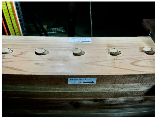
Figure 21. Protruding wooden A-type dowel.
