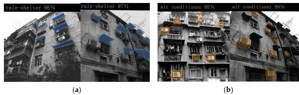
Figure 9. Automated recognition for spontaneous space for assisted living form. Present situation identification of rain-shelter (a); present situation identification of air conditioner (b).
