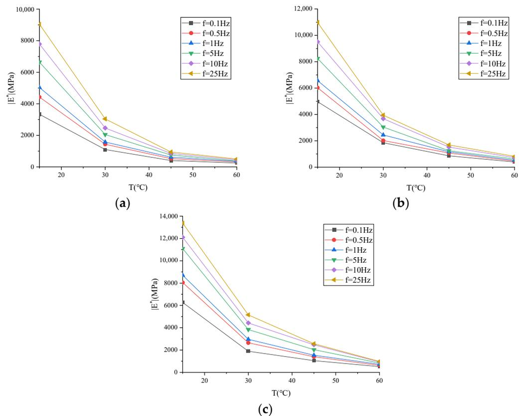
**Figure 10.** Variation trends of dynamic moduli of asphalt mixtures with temperature: (a) ARHM-13; (b) ARHM-20; (c) ARHM-25.
