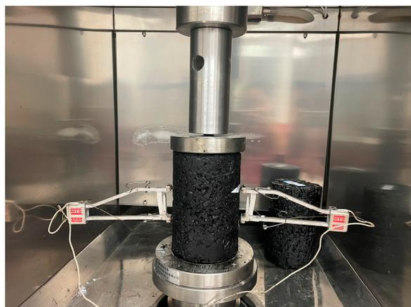
**Figure 1.** Dynamic modulus testing under uniaxial compression conditions.
