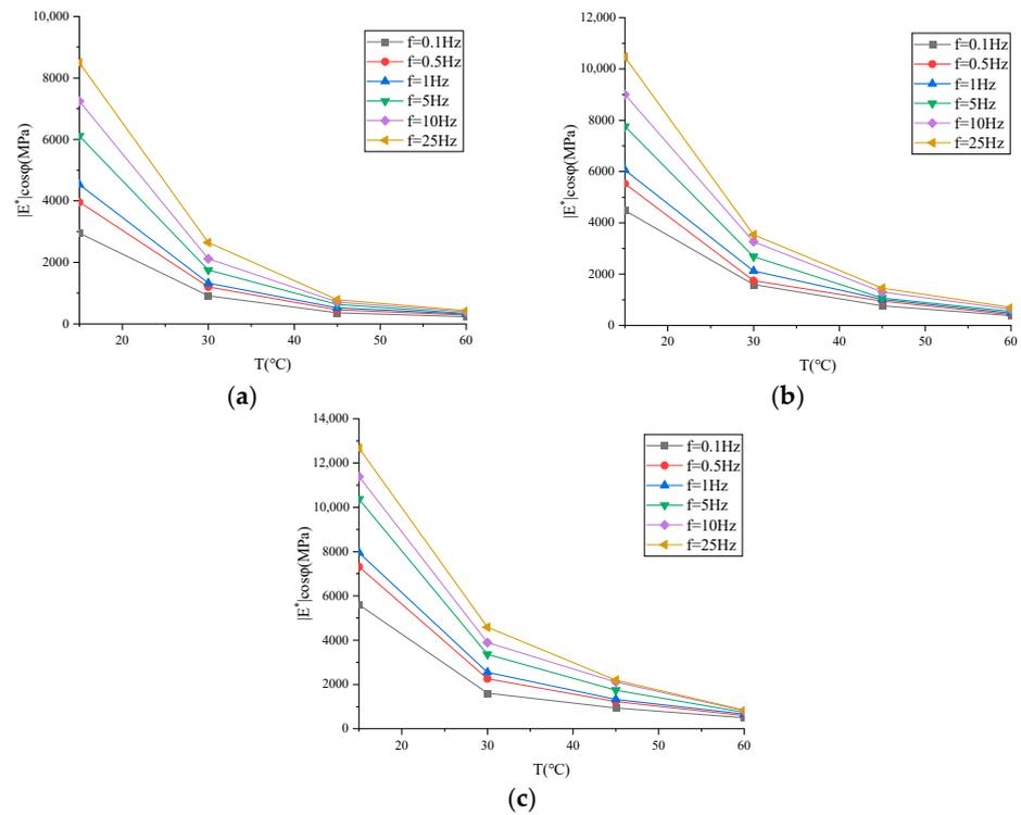
**Figure 12.** Variation trend of storage modulus of asphalt mixture with temperature: (a) ARHM-13; (b) ARHM-20; (c) ARHM-25.
