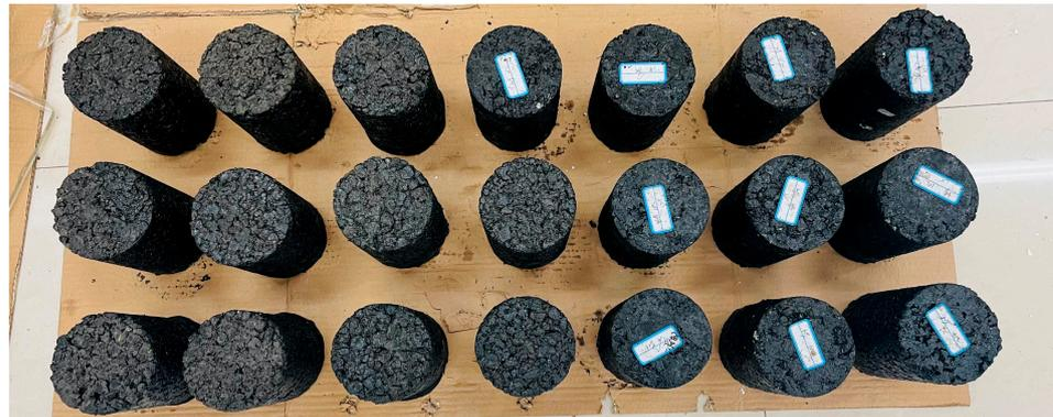
**Figure 3.** Asphalt mixture specimens.
