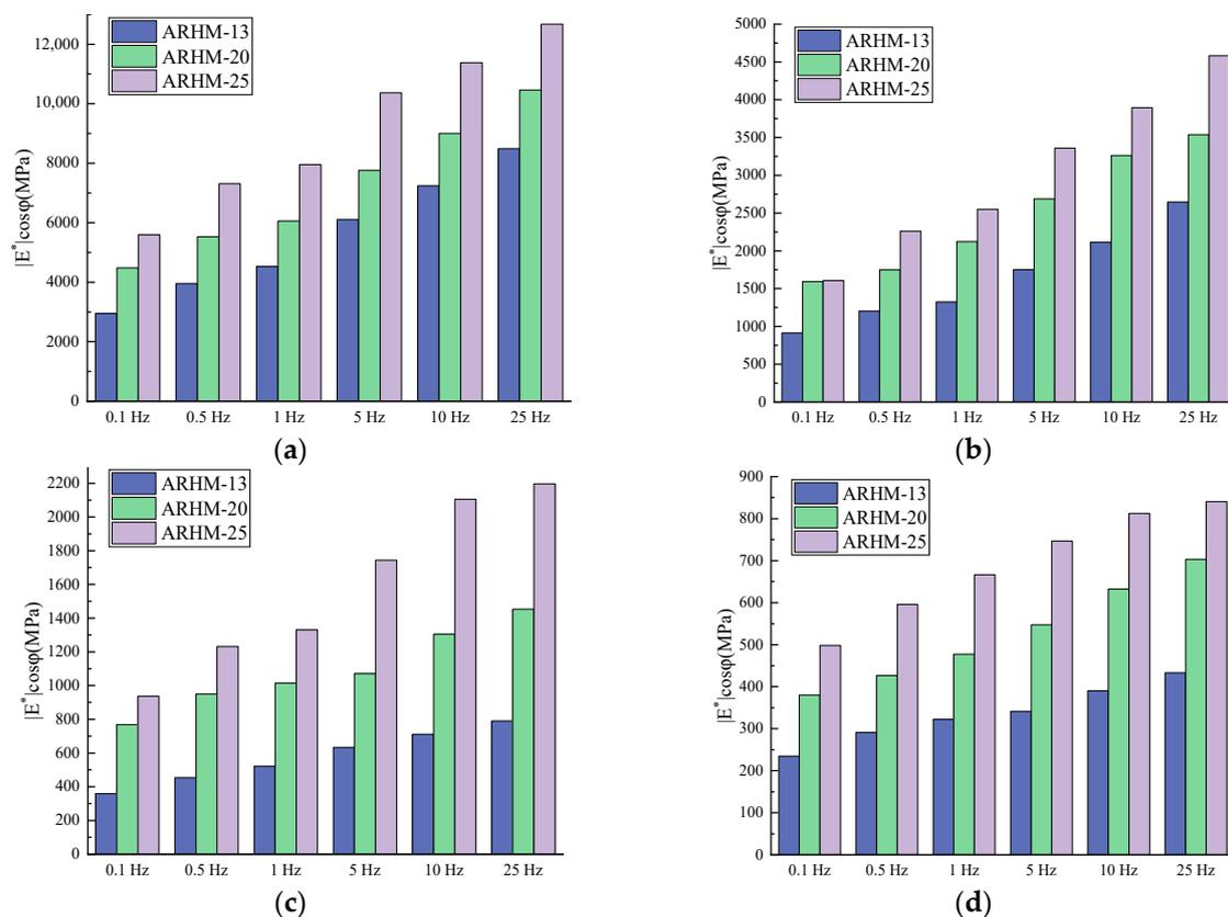
**Figure 18.** Relationship between asphalt mixture type and storage modulus: (a)  $T = 15^\circ\text{C}$ ; (b)  $T = 30^\circ\text{C}$ ; (c)  $T = 45^\circ\text{C}$ ; (d)  $T = 60^\circ\text{C}$ .
