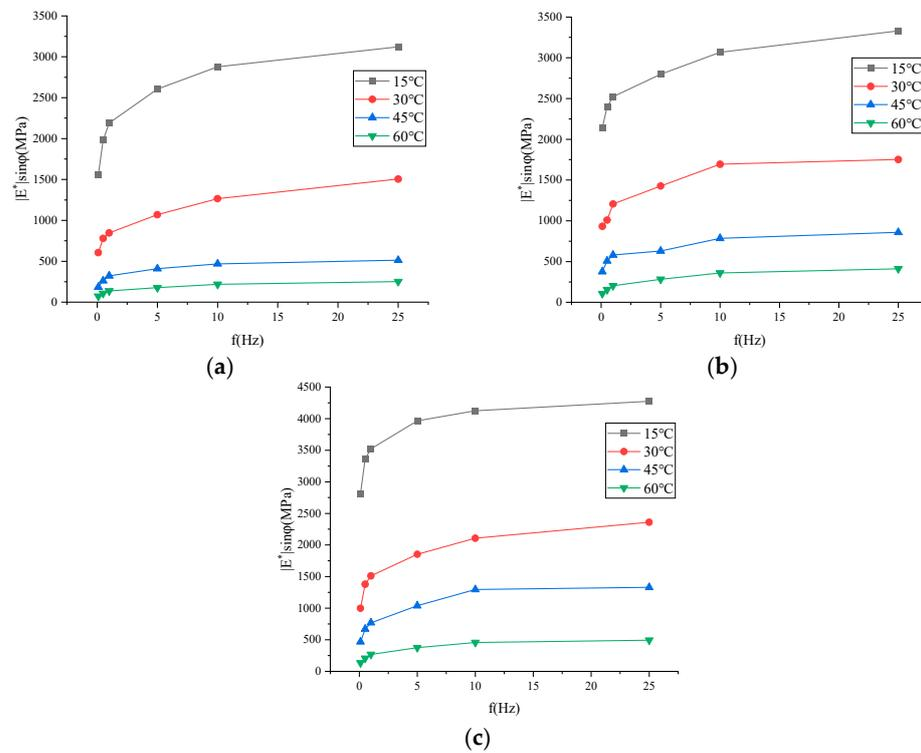
**Figure 7.** Variation trend of asphalt mixture loss moduli with loading frequency: (a) ARHM-13; (b) ARHM-20; (c) ARHM-25.
