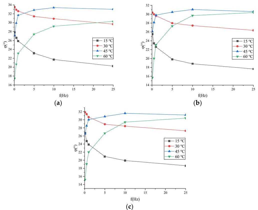
**Figure 5.** Variation trend of phase angle of asphalt mixtures with loading frequency: (a) ARHM-13; (b) ARHM-20; (c) ARHM-25.
