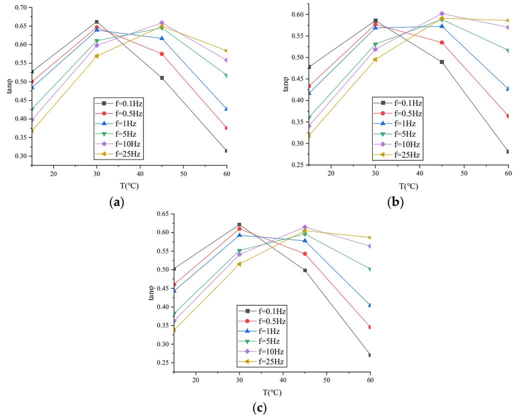
**Figure 14.** Variation trend of asphalt mixture loss factors with temperature: (a) ARHM-13; (b) ARHM-20; (c) ARHM-25.
