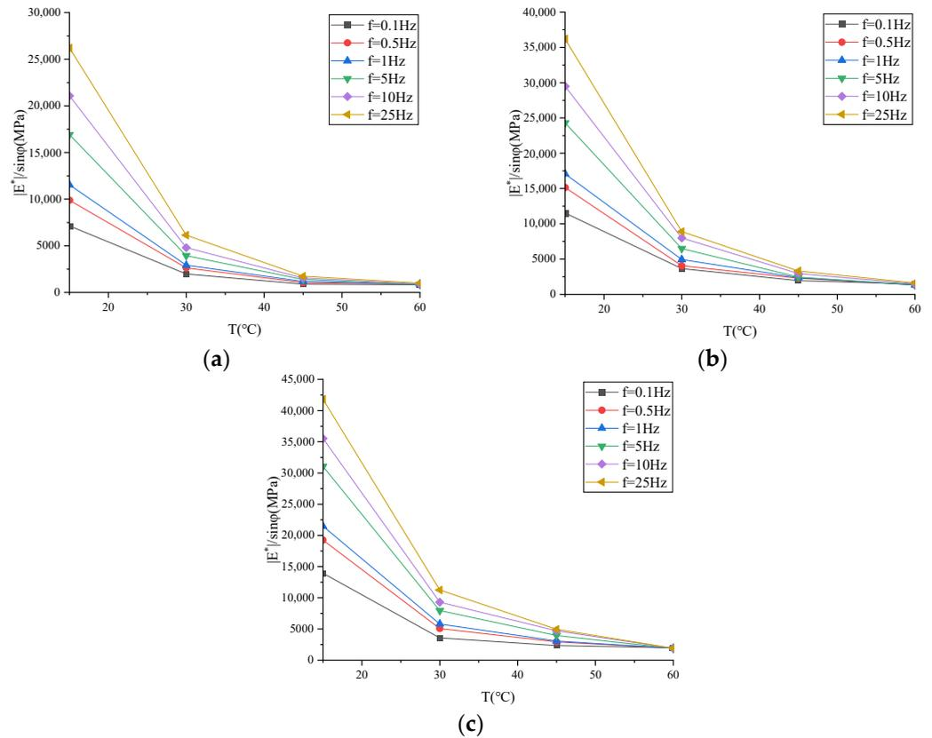
**Figure 15.** Trend of rutting factors of asphalt mixtures with temperature: (a) ARHM-13; (b) ARHM-20; (c) ARHM-25.
