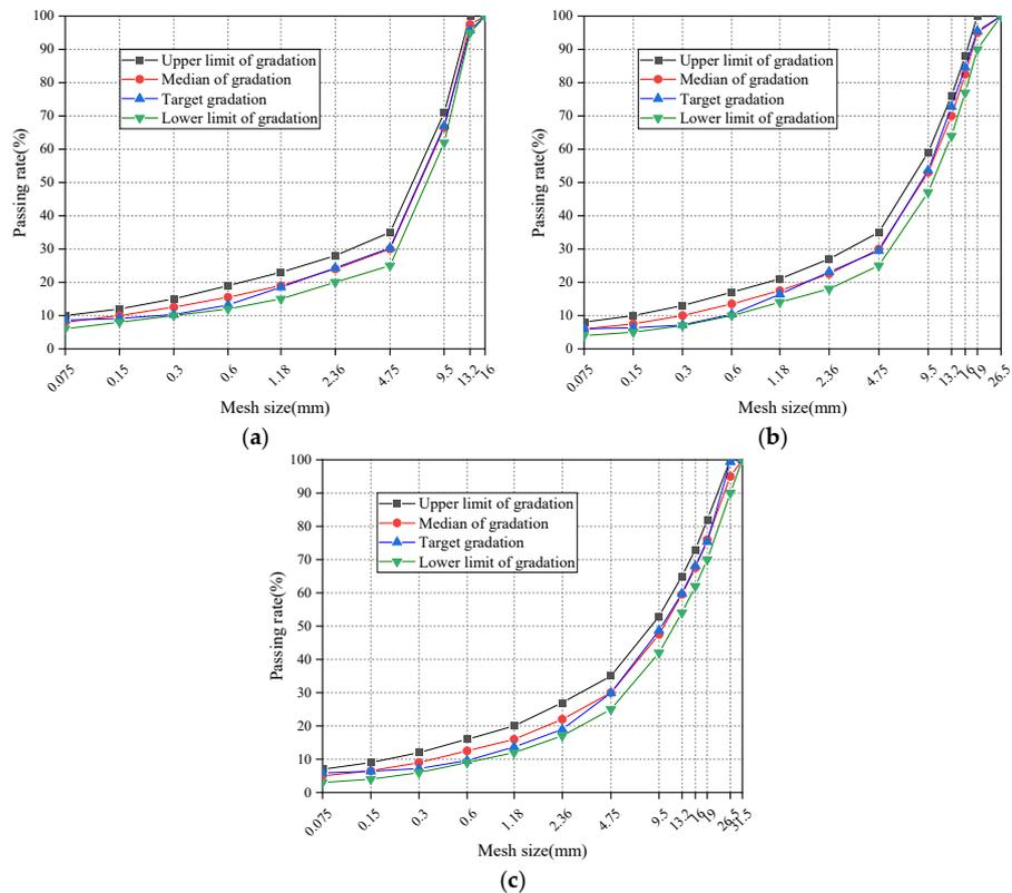
**Figure 2.** Asphalt mixture mineral grading curve: (a) ARHM-13; (b) ARHM-20; (c) ARHM-25.
