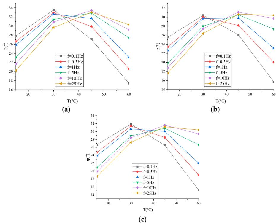
**Figure 11.** Variation trends in phase angles of asphalt mixtures with temperature: (a) ARHM-13; (b) ARHM-20; (c) ARHM-25.
