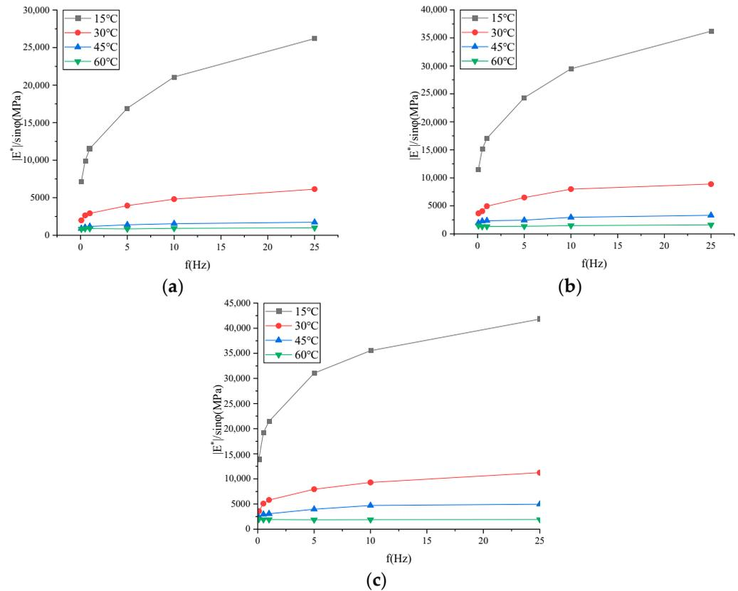
**Figure 9.** Trends in the rutting factors of asphalt mixtures with loading frequency: (a) ARHM-13; (b) ARHM-20; (c) ARHM-25.
