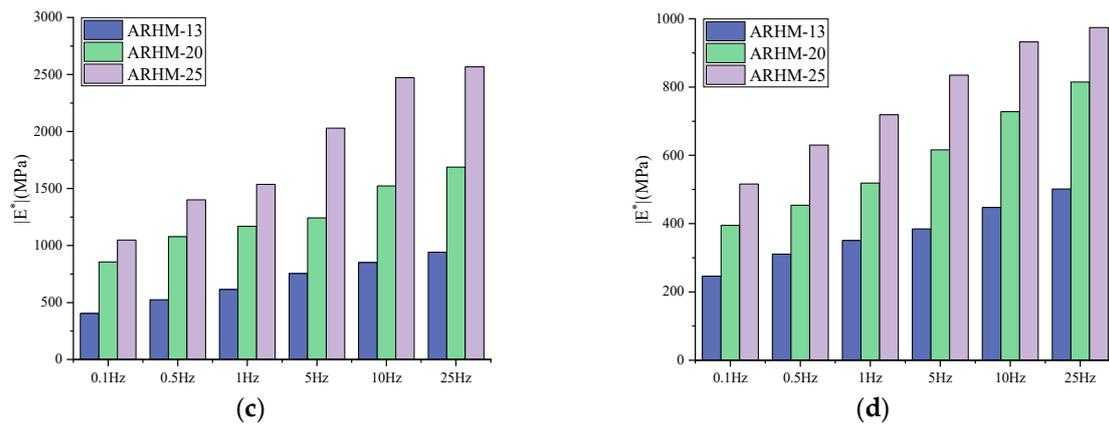
**Figure 16.** Relationship between type of asphalt mixture and dynamic modulus: (a)  $T = 15^\circ\text{C}$ ; (b)  $T = 30^\circ\text{C}$ ; (c)  $T = 45^\circ\text{C}$ ; (d)  $T = 60^\circ\text{C}$ .
