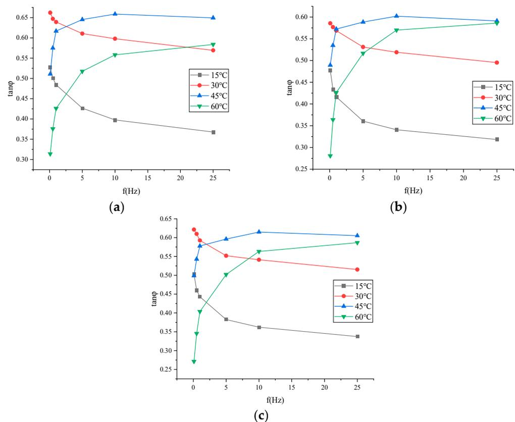
**Figure 8.** Variation trend of asphalt mixture loss factors with loading frequency: (a) ARHM-13; (b) ARHM-20; (c) ARHM-25.
