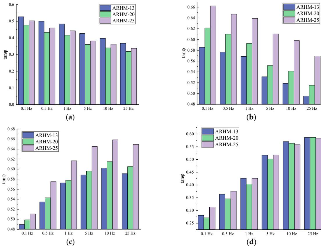
Figure 20. Relationship between asphalt mixture type and loss factor: (a) T = 15 °C; (b) T = 30 °C; (c) T = 45 °C; (d) T = 60 °C.
