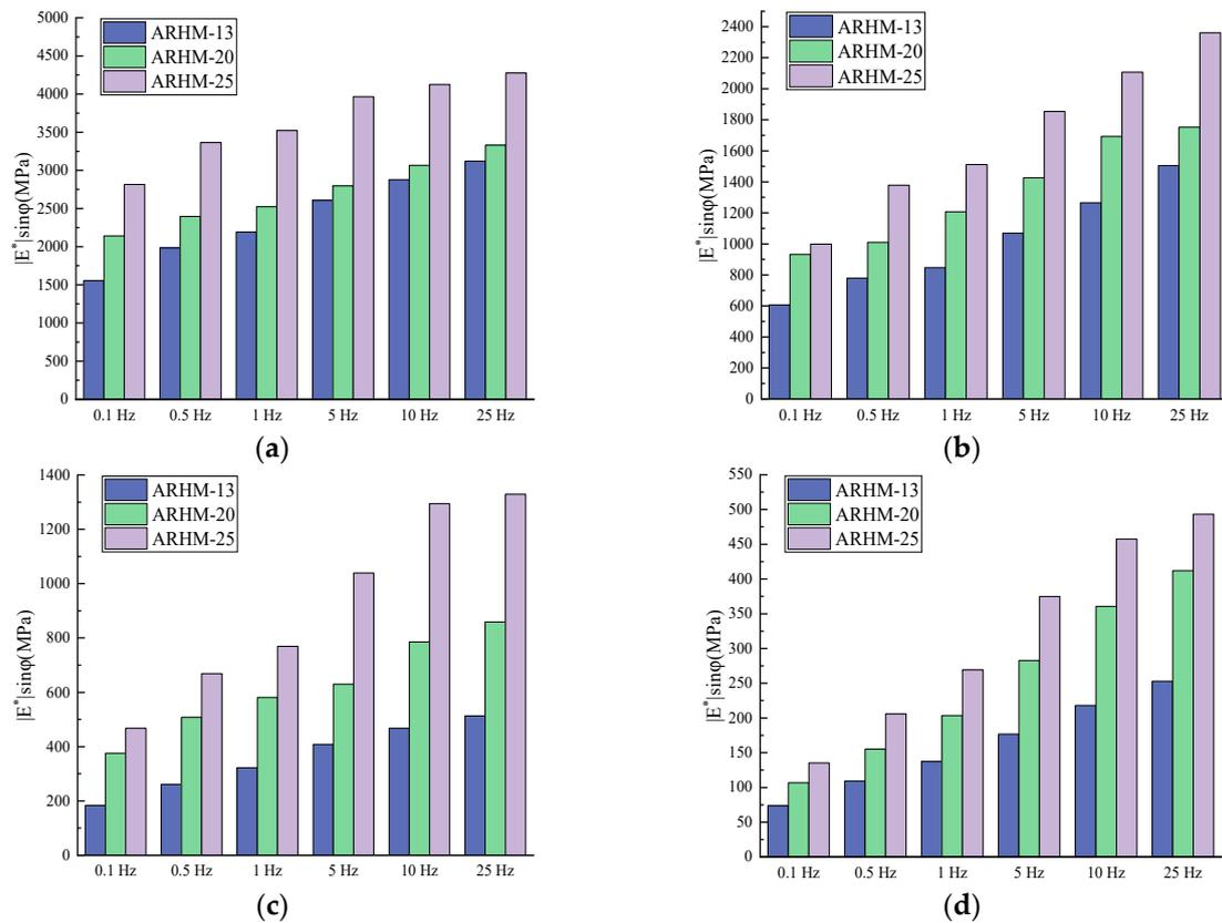
**Figure 19.** Relationship between asphalt mixture type and loss modulus: (a)  $T = 15\text{ }^{\circ}\text{C}$ ; (b)  $T = 30\text{ }^{\circ}\text{C}$ ; (c)  $T = 45\text{ }^{\circ}\text{C}$ ; (d)  $T = 60\text{ }^{\circ}\text{C}$ .
