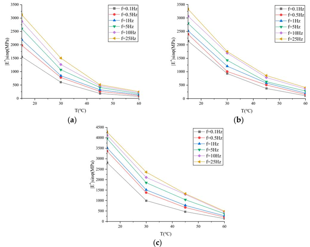
**Figure 13.** Variation trend of loss moduli of asphalt mixtures with temperature: (a) ARHM-13; (b) ARHM-20; (c) ARHM-25.
