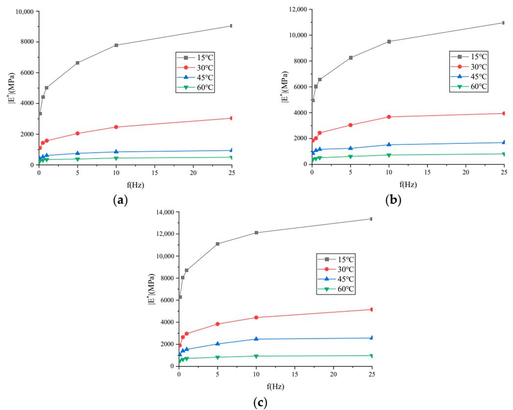
**Figure 4.** Variation trend of dynamic modulus of asphalt mixture with loading frequency: (a) ARHM-13; (b) ARHM-20; (c) ARHM-25.
