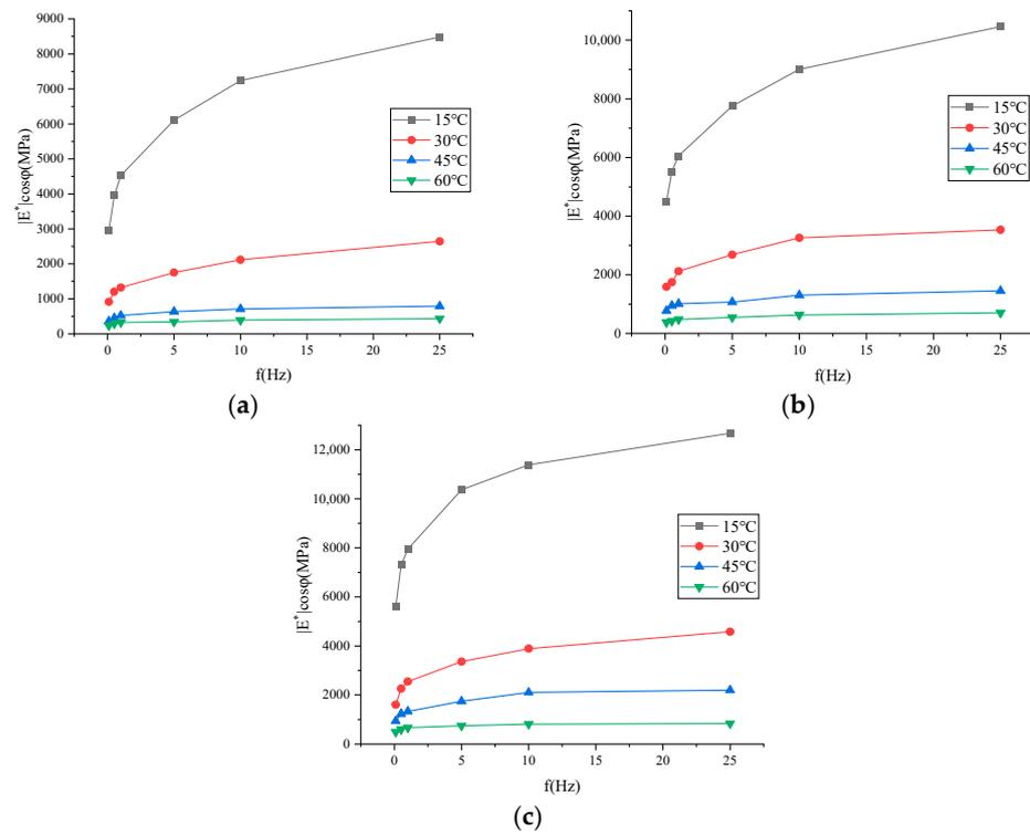
**Figure 6.** Variation trend of storage moduli of asphalt mixture with loading frequency: (a) ARHM-13; (b) ARHM-20; (c) ARHM-25.
