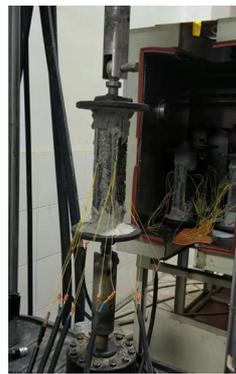
Figure 20. Tensile test loading process.
