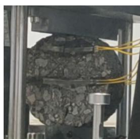
**Figure 9.** Starting state of the 19 mm arc bead splitting end face.
