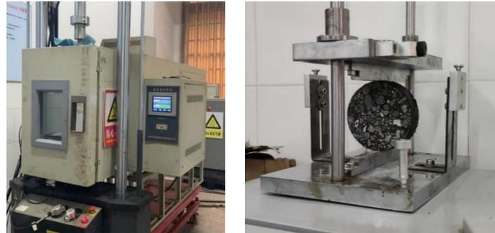
**Figure 3.** Example of specimen splitting and loading.
