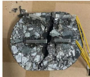
**Figure 12.** Splitting failure state of the rigid pressing plate.
