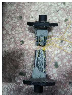
Figure 21. Specimen after loading for the tensile test.
