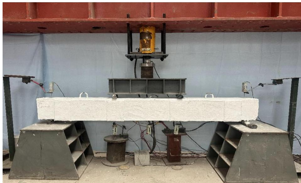
**Figure 7.** Beam loading device diagram. (a) Schematic diagram of loading device; (b) loading device on-site diagram.
