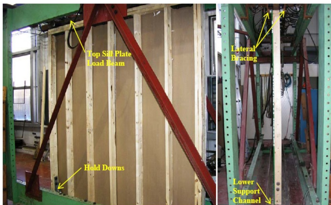
Figure 3. Shearwall test frame with specimen installed.
