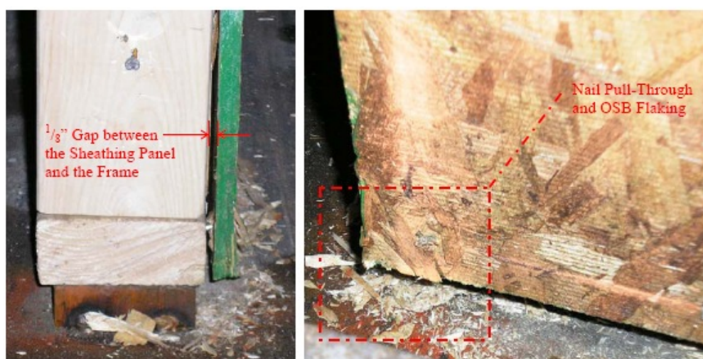
Figure 15. Nail pull-through along the center stud.
