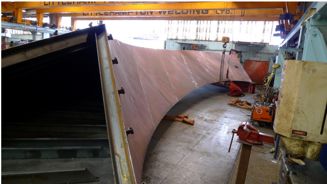
Figure 27. Assembly of one segment. This is 18 m long and the full sculpture consists of eleven different segments.
