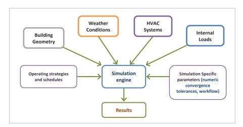
**Figure 1.** General input data of thermal simulation engines [5].
