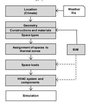
**Figure 4.** An ideal workflow for energy performance in thermal simulation tools [5].
