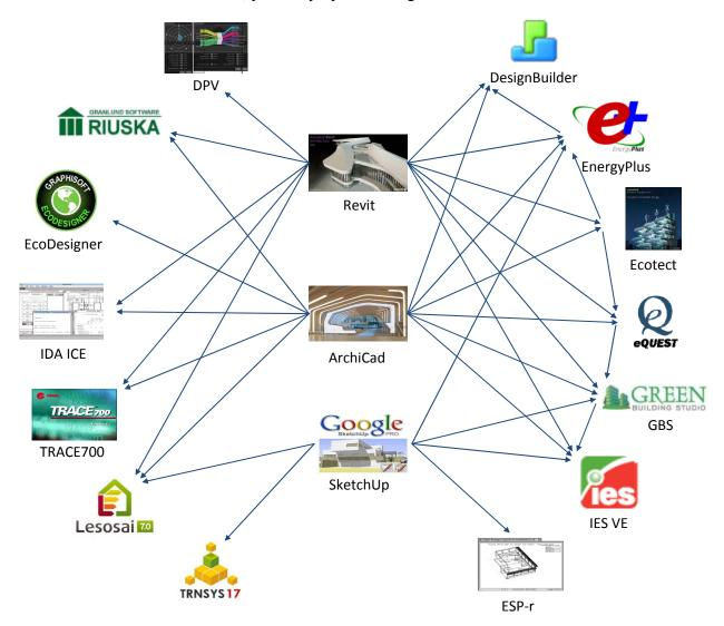
ArchiCAD is an architectural BIM/CAD tool supplied by Graphisoft/Abvent. EcoDesigner is built into ArchiCAD as an interface. The ArchiCAD BIM program also links with Design Builder, Ecotect, EnergyPlus, Green Building Studio, Lesosai, TRNSYS, IDA ICE, IES VE, TRACE700, and Riuska. Within ArchiCAD, it is possible to create zones and then export the simplified energy model into Ecotect using Green Building Studio's .gbXML format, where the energy analysis and solar design can be completed.
