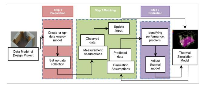
Figure 2. Workflow to produce a thermal simulation model.
