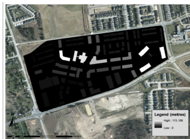
Figure 3. Original site plan design—converted 2D raster digital elevation model (DEM) at a resolution of 0.5 m converted from 3D file, projected onto orthophoto.
