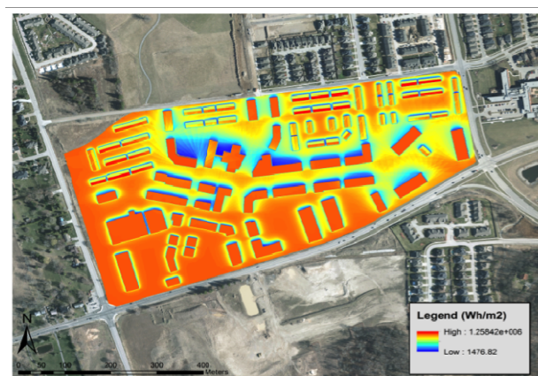
Figure 5. Example of an annual solar insolation map generated from the methodology for the original site plan.
