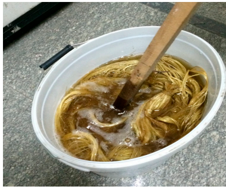
Figure 2. Submerging banana fibers in NaOH solution.
