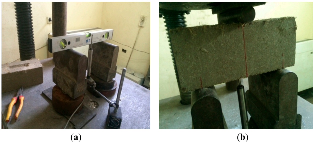
Figure 7. (a) Leveling the two supports and centering Linear Variable Differential Transformer (LVDT); (b) Flexural strength test set-up.
