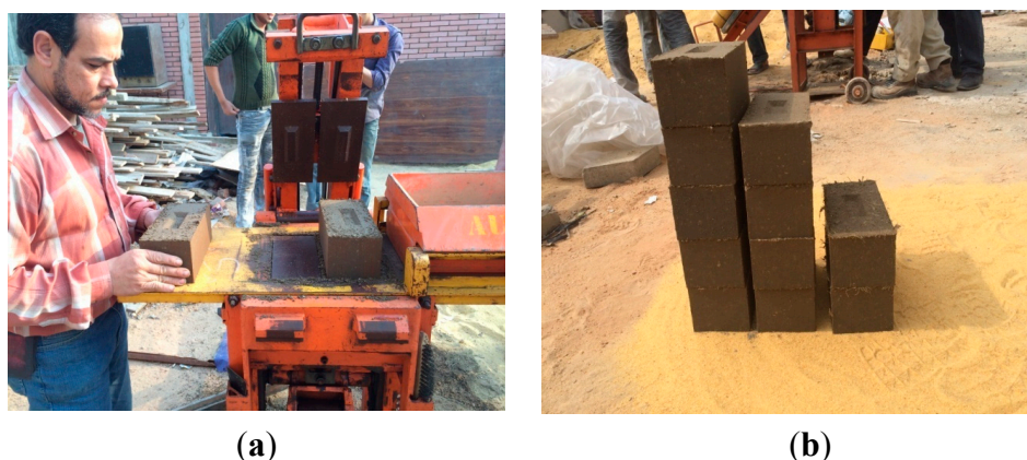
Figure 4. (a) Ejecting the Green-Compressed Earth Block (GCEB) from the mold; (b) Placing the blocks outdoors.
