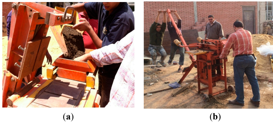
Figure 3. (a) Filling the mold with the mix using a bucket; (b) Manual pressing using Compressed Earthen Block (CEB) machine.
