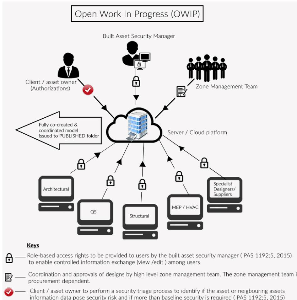
**Figure 7.** Information exchange and access control in OWIP.
