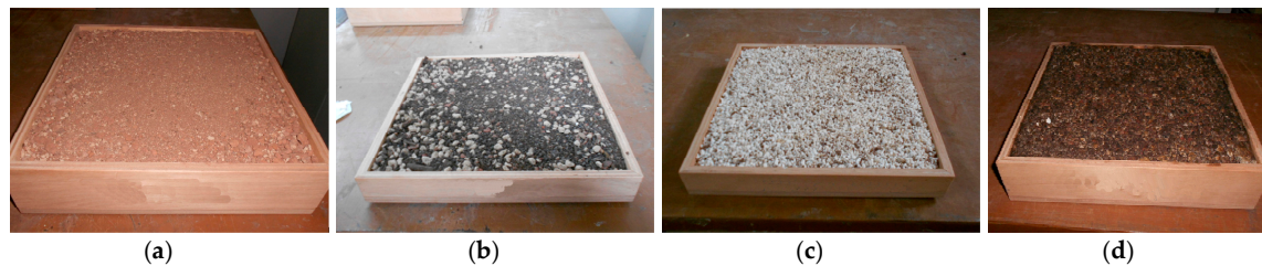
Figure 1. Extensive samples inserted in the relevant containment systems, ready for the thermal flow meter method tests; (a) Factory 1, (b) Factory 2, (c) Factory 3, (d) Factory 4.
