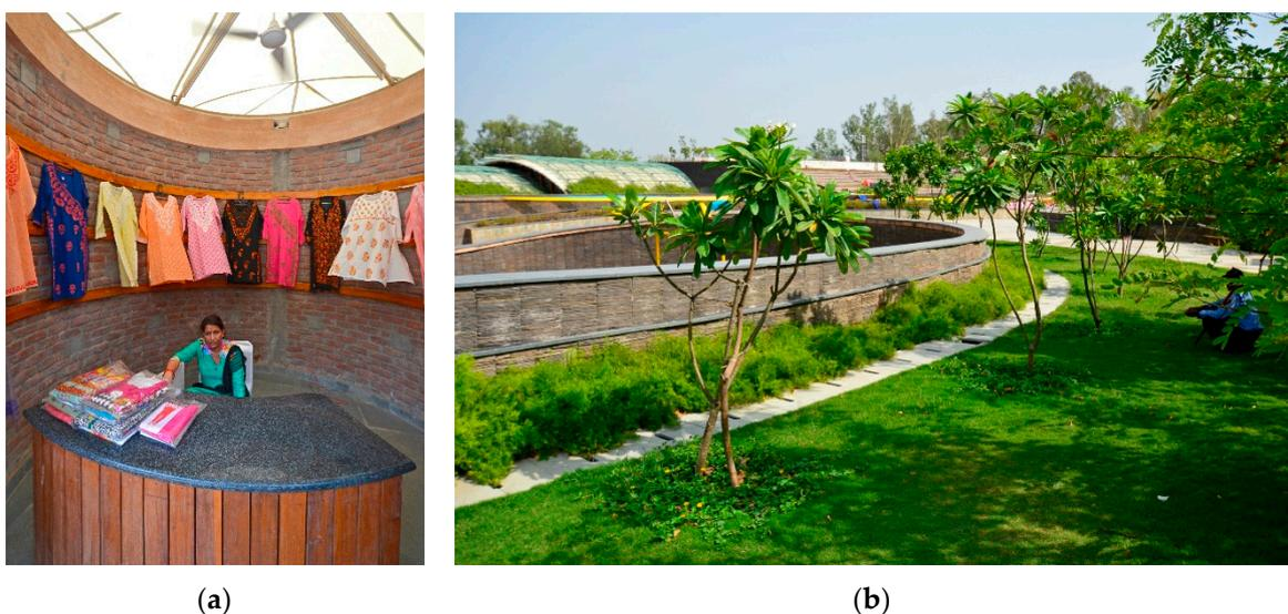
**Figure 34.** (a) Tensile canopies with ceiling fans cover the craft shops; (b) large usable green roofs above air-conditioned shops (Photos: Author).
