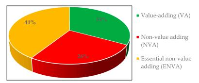
Figure 6. Average of each activity classification type for all observed construction processes.
