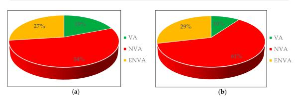
**Figure 1.** Summary of the VSM data of the process "installation of floor slab" (**a**) for person 1—crane operator, (**b**) for persons 2 and 3—installation workers.
