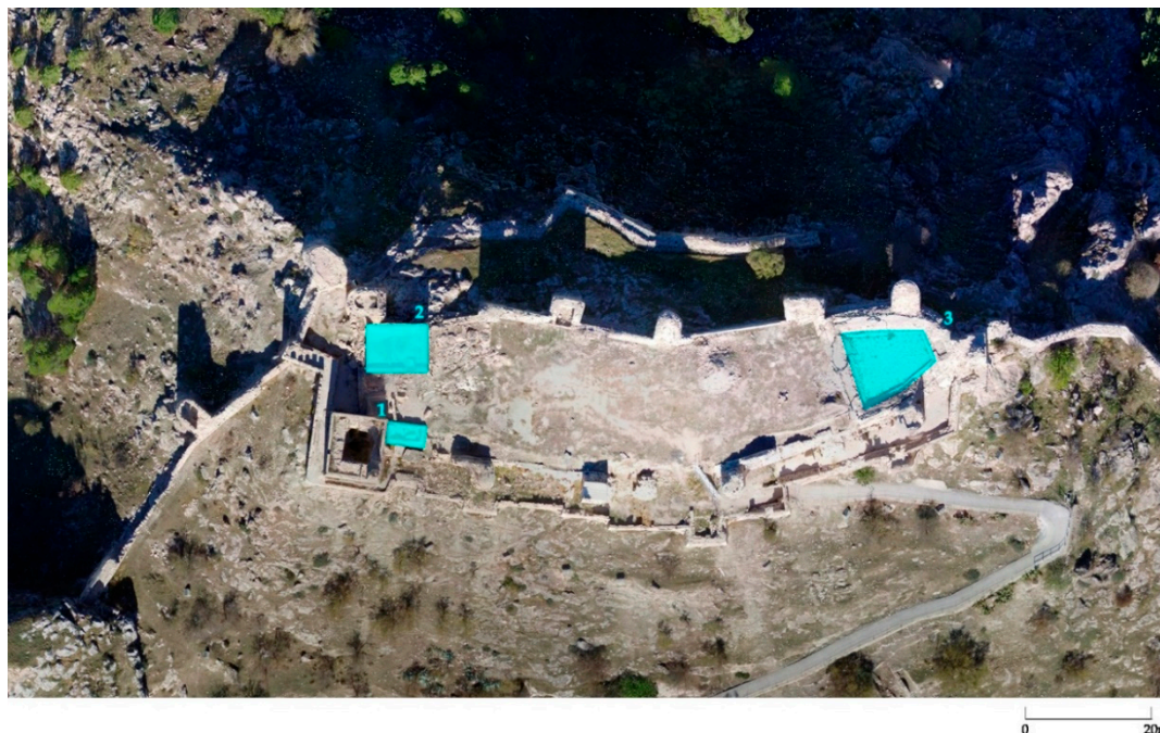
Figure 11. Orto-corrected photogrammetry of the Alcazaba of Moclín. Isolated hydraulic constructions: (1) Oldest cistern, (2) large cistern, and (3) possible collection surface. Created by authors.
