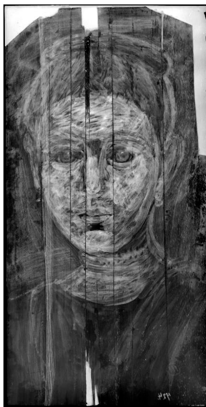
Figure 6. X-radiograph of the Girl with the Golden Wreath; technical specifications: 25 kV, 2 mA, 60 s, 100 cm. [Image credit: Judith van der Brugge-Mulder; edited for brightness and contrast by Jan van Daal].
