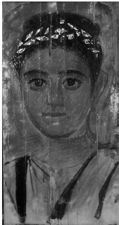
Figure 7. OSIRIS infrared reflectogram of the panel portrait taken at a wavelength of 0.9–1.7 \mu\text{m} . [Image credit: Moorea Hall-Aquitania; edited by Jan van Daal].
