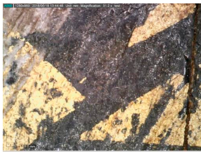
Figure 8. Micrograph of the intersection of three gilded leaves taken at 29 \times magnification from the golden wreath in the girl's hair. [Image credit: Jan van Daal].
