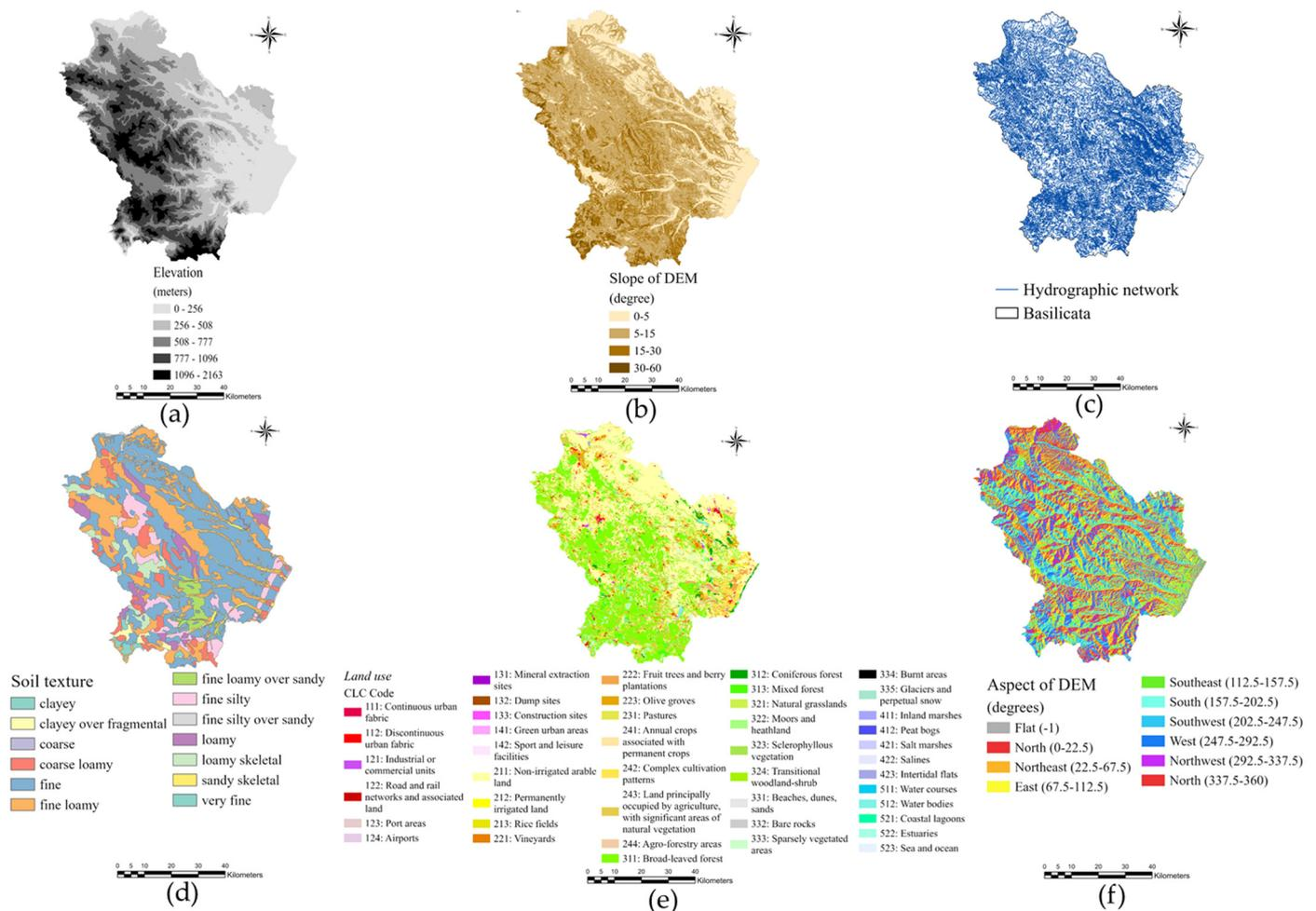
**Figure 9.** Environmental data-layers selected for GIS model construction: (a) Elevation; (b) Slope; (c) Hydrographic network; (d) Soil texture; (e) Land use; (f) Aspect.
