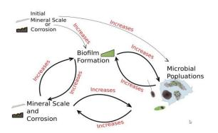
**Figure 10.** A horrible synergy—Control of scale and corrosion is part of microbial control. (Figure 10 generated by Daniel Brouse).
