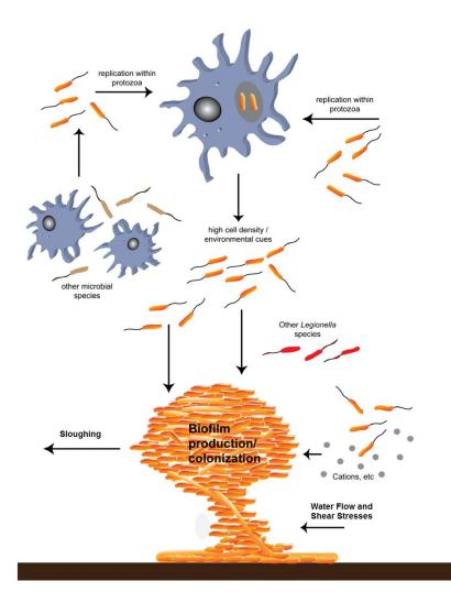
**Figure 9.** Biofilm formation-*Legionella* parasitic infestation of protozoa and effects of water flow on sloughing and redistribution of planktonic *L. pneumophila* in cooling water systems. (Image modified from [9]).
