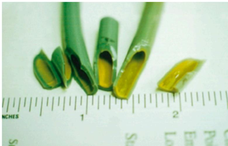
**Figure 2.** Biofilm formation on dental unit waterline tubing (reproduced with permission from Mills SE [41]).
