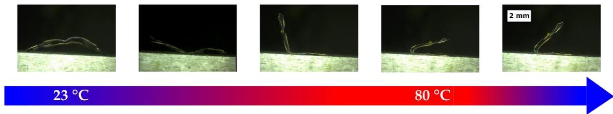
**Figure 5.** Folding sequence of a mechanically deformed SMA folding microactuator at room temperature. The memory shape can be recovered by heating on a hot plate above the austenite finish temperature.
