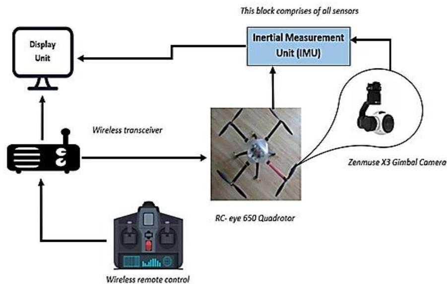
Figure 23. Block diagram demonstrating the experimental setup.
