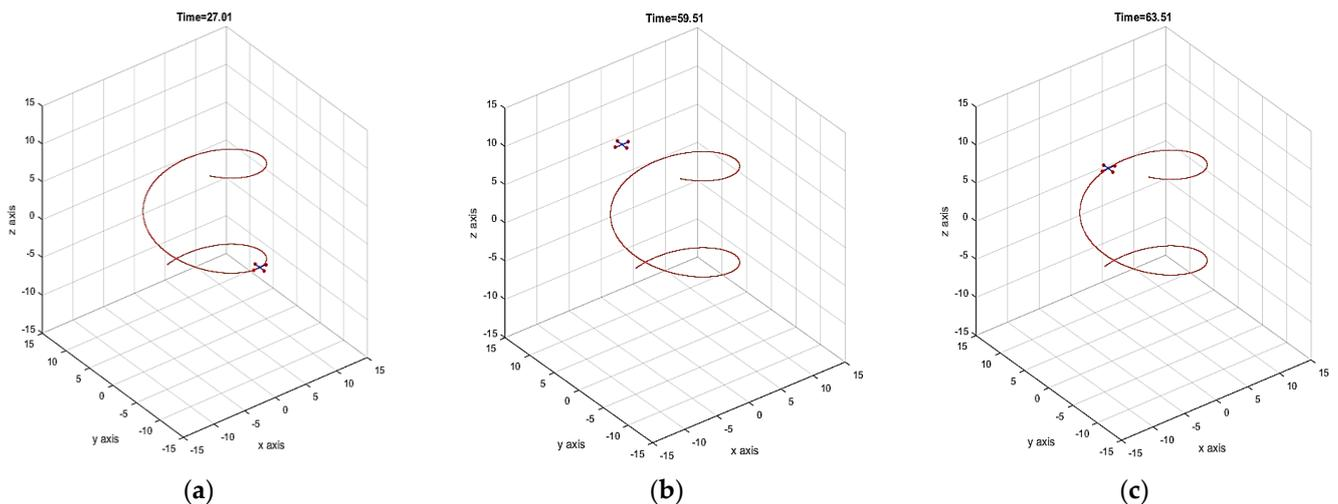
Figure 12. Quadrotor following helical trajectory using F-SMC control design.
