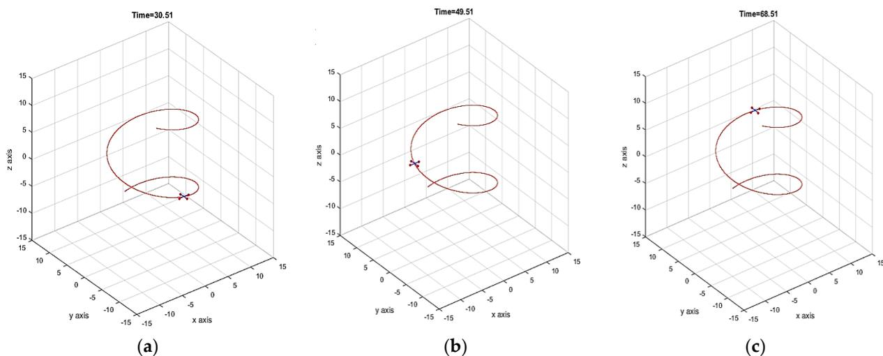
**Figure 18.** Quadrotor following helical trajectory using MFSDF-SMC control design.
