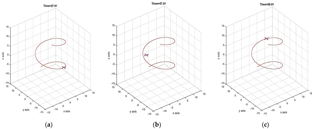
**Figure 17.** Quadrotor following helical trajectory using SDF-SMC (without model-free approach).
