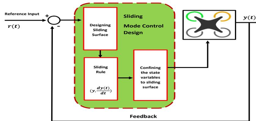
Figure 5. Block diagram for fuzzy-based sliding mode control (FSMC).
