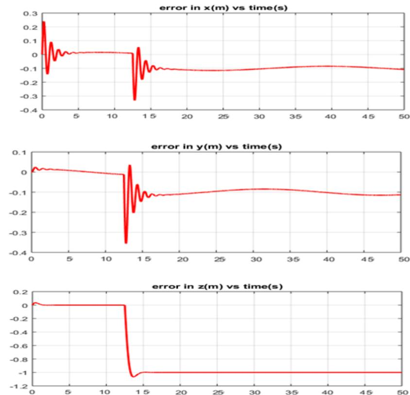
**Figure 21.** Position error rates while maneuvering using MFSDf-SMC.
