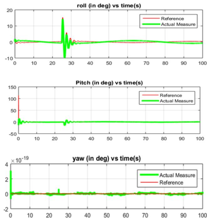
Figure 14. Roll, pitch and yaw response using F-SMC control technique.
