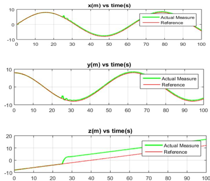
**Figure 10.** Position responses derived using SMC control technique.
