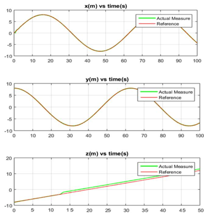
Figure 13. Position response derived using F-SMC control technique.
