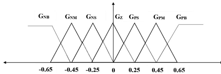
Figure 8. New revised input membership functions based on variable G.
