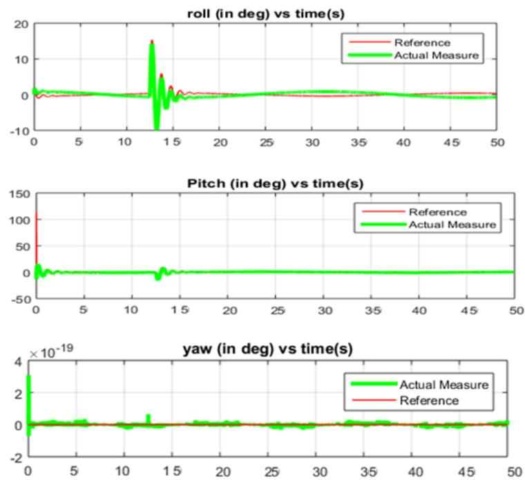
Figure 16. Roll, pitch and yaw responses using SDF-SMC control technique.
