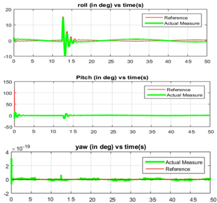
Figure 20. Roll, pitch and yaw responses using SDF-SMC control technique.
