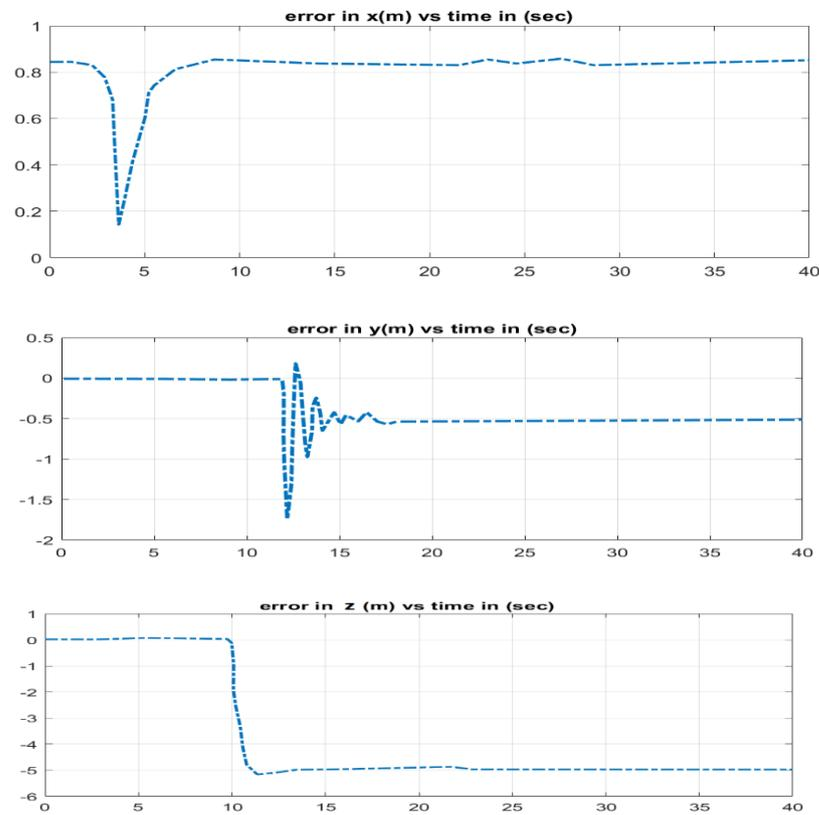
**Figure 24.** Position error rates while maneuvering using MFSDF-SMC during hardware implementation.
