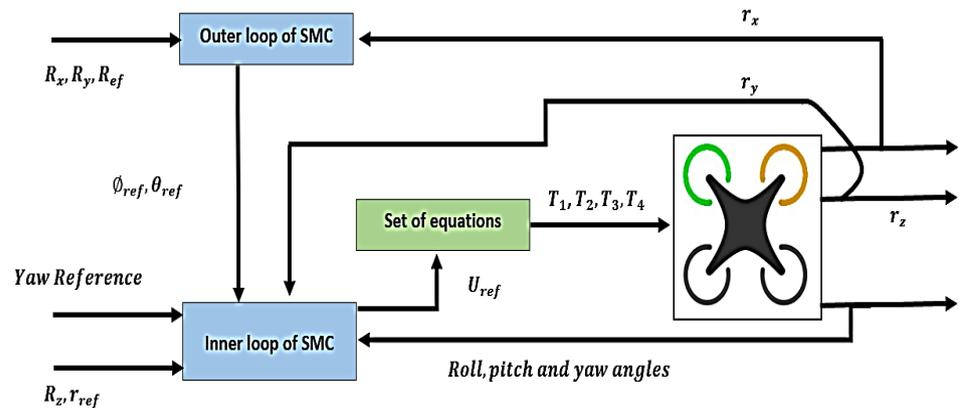
Figure 1. Conventional block diagram of SMC.
