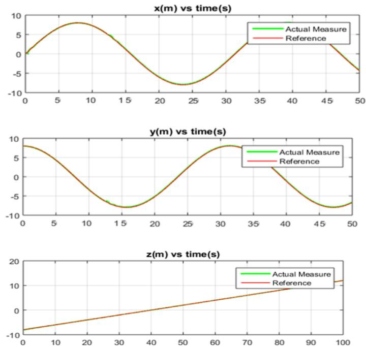
Figure 15. Position response derived using SDF-SMC control technique.
