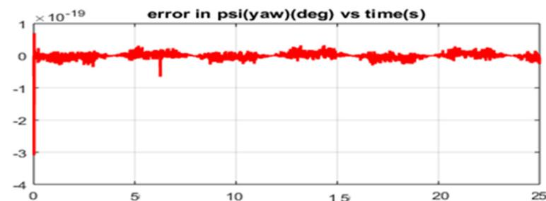
**Figure 22.** Yaw error rates while maneuvering using MFSDf-SMC.
