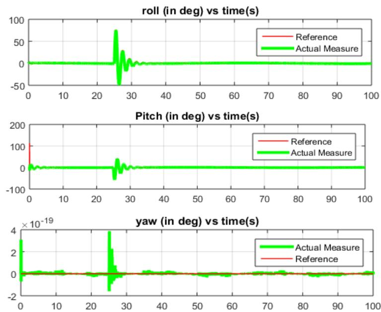
Figure 11. Roll, pitch and yaw responses using SMC Control technique.
