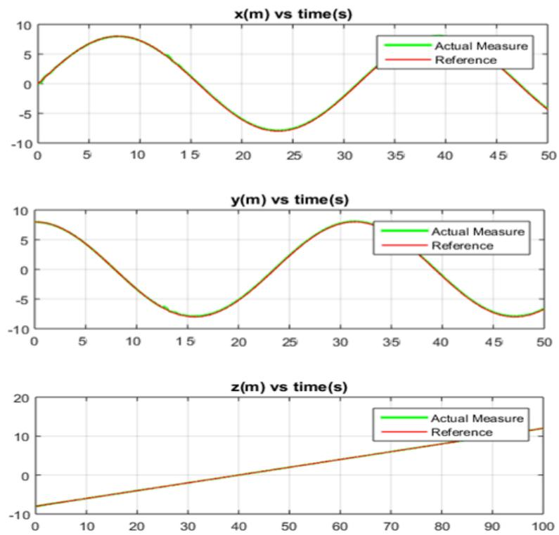
Figure 19. Position response derived using SDF-SMC control technique.
