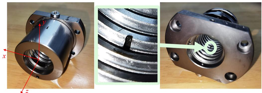
Figure 16. Faulty nut used in the EMA test stand.
