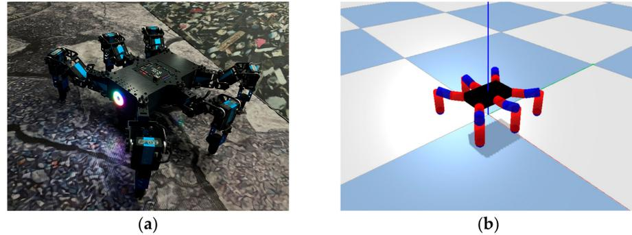
**Figure 1.** (a) Physical prototype of the hexapod robot VkHex; (b) simulated prototype of the VkHex in PyBullet.
