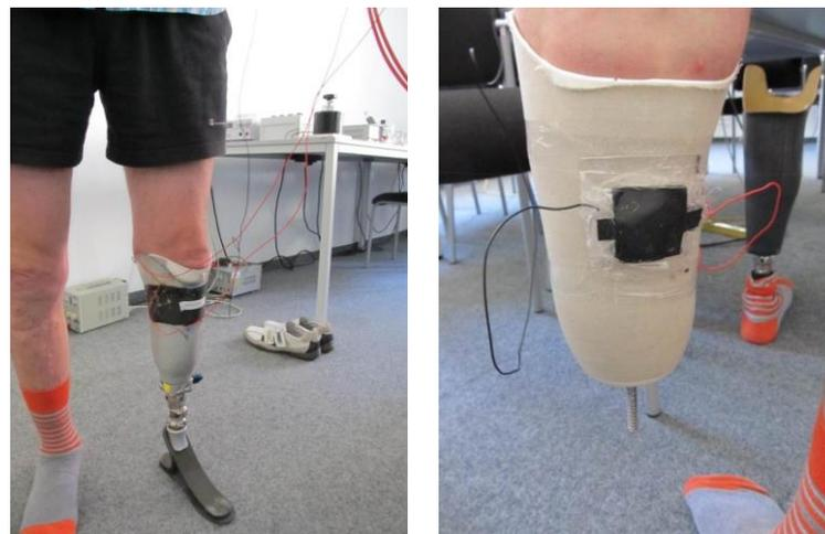
**Figure 19.** DE pressure sensor attached on the liner of a knee prosthesis for an experimental evaluation [100].
