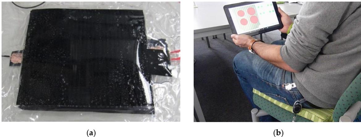
**Figure 18.** DE pressure sensor for seat applications (a) and demonstration of monitoring the weight distribution of a person on a chair cushion with four sensors (b) [100].
