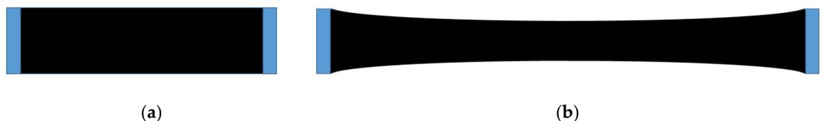
**Figure 2.** Scheme of a dielectric elastomer strain sensor (a) that is stretched with transversal contraction (b).
