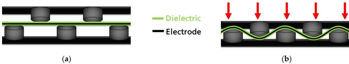
**Figure 9.** Scheme of a dielectric elastomer pressure sensor with two knot-shaped profiled outer films with electrode layers and an elastomer film with only one electrode layer covered by two dielectric layers between the profiles in the unloaded state (a) and in the loaded state (b) [99].
