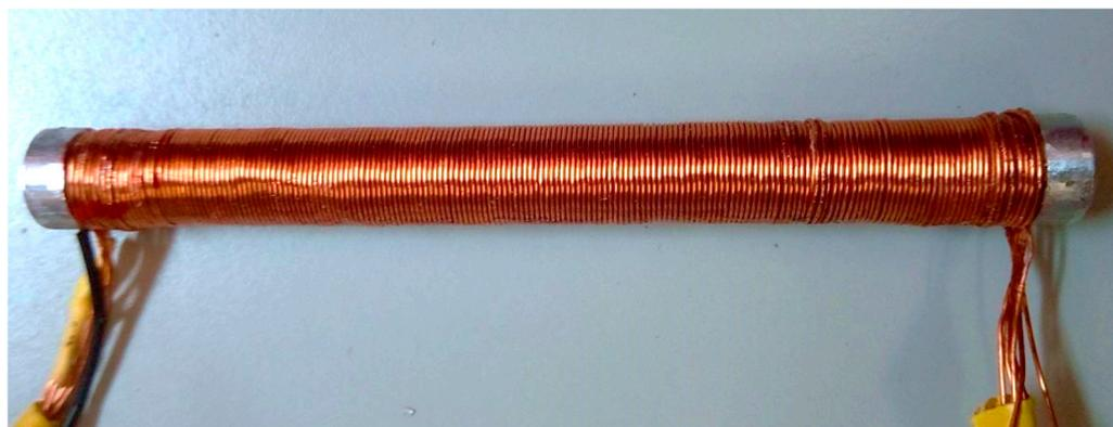
**Figure 4.** Manufactured magnetorquer prototype.
