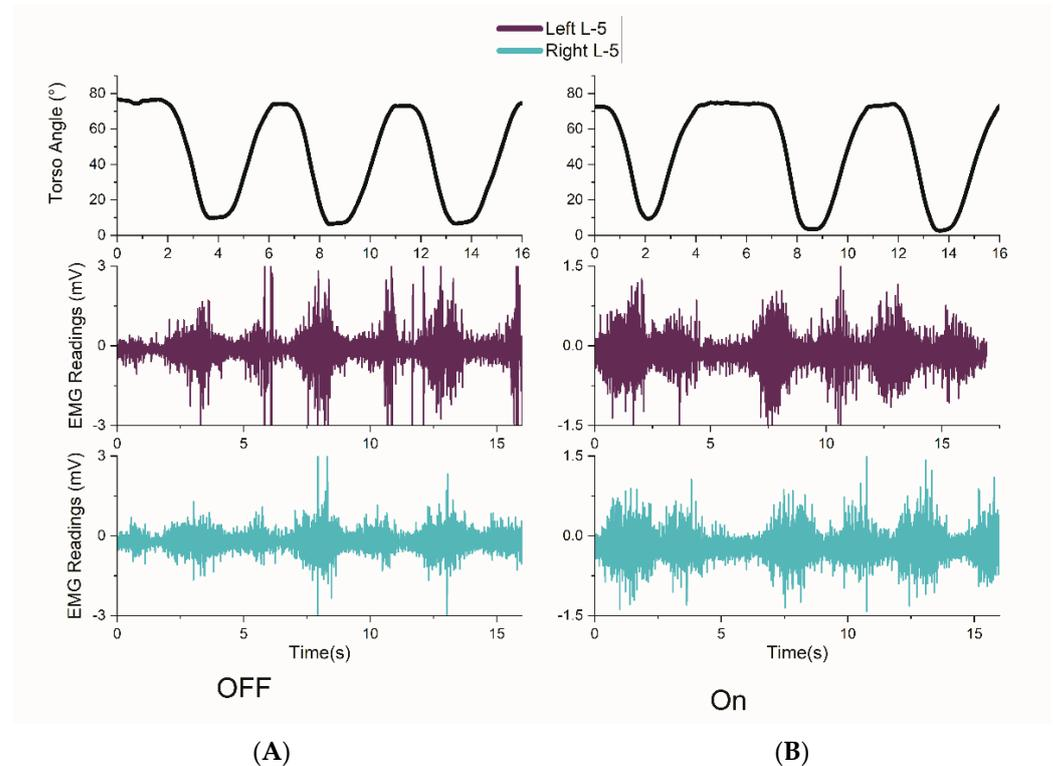
**Figure 6.** Time series data showing a subject's torso angle and Raw EMG readings on the Lumbar-5 region for one 20 kg set. At a 90° torso angle, the torso is fully flexed. (A) Unpowered. (B) Powered.
