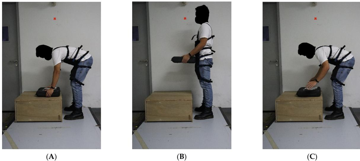
**Figure 4.** The supported lifting motion is shown. (A) Sets start in the flexed position. (B) The container is raised to the standing position (C) and is returned to the flexed position. The user is instructed to release the container.
