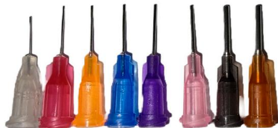
**Figure 2.** Suction needles with inner diameters of 0.21, 0.26, 0.33, 0.41, 0.51, 0.6, 0.65 and 0.84 mm were used for experiments.
